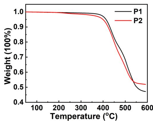
**Fig. S1.** TGA curves of P1 and P2.
