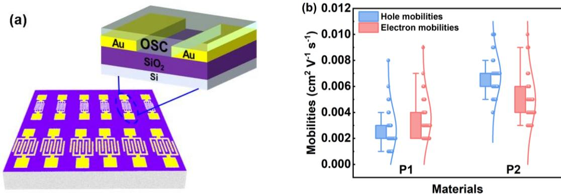
**Fig. S23.** (a) Schematic diagram of BGBC type OFETs. (b) Statistical distribution diagram of hole and electron mobilities of P1 and P2 with 30 devices, respectively. The box chart ranges within 1.5 quartile.
