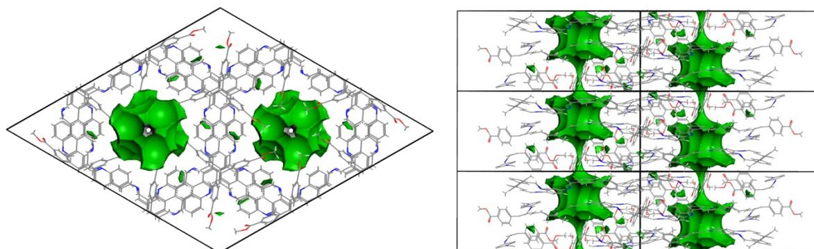
Figure S 4: Solvent accessible surfaces of the two central pores in the **4A2E**-PDA-COF with a 1.4  $\text{\AA}$  Probe radius viewed along the [001] direction (left) and the [110] direction (right). Symmetry equivalent pores at the unit cell boundary were omitted for clarity.
