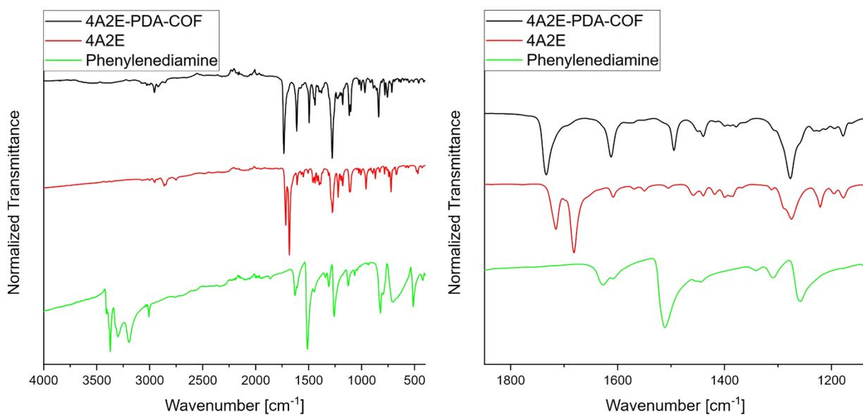
Figure S 6: IR of **4A2E**-PDA-COF (black), **4A2E** linker (red) and Phenylenediamine (green).
