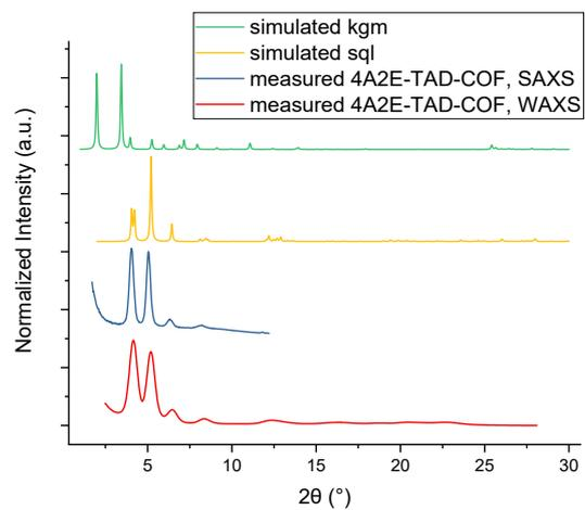
Figure S 15: PXRD measurement of the 4A2E-TAD-COF in small and wide angle configuration. Comparison with simulated *kgm* and *sql* PXRD spectra.
