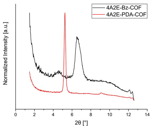
Figure S 12: PXRD measurement of the **4A2E**-PDA-COF and **4A2E**-Bz-COF in the small angle configuration.
