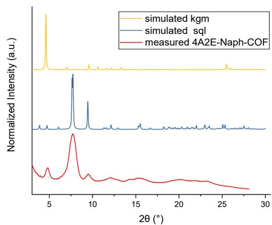
Figure S 13: PXRD measurement of the 4A2E-Naph-COF in wide angle configuration. Comparison with simulated *kgm* and *sql* PXRD spectra.
