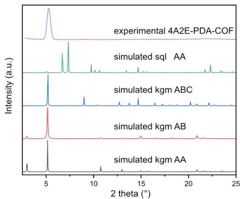
Figure S 5: PXRD comparison **4A2E**-PDA-COF with *sql* AA, *kgm* ABC, *kgm* AB and *kgm* AA stacking.
