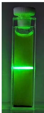
**Fig. S27:** Digital image of Tyndall effect exhibited by IPcomp-8 in aqueous medium.
