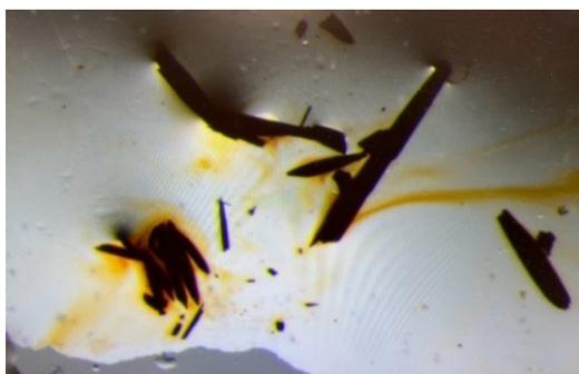
Figure S4. Crystals of **P6-III** and **P6-IV** dissolve shortly (<20 sec) after contact with Paratone oil. For scale, the width of the large plate is ca. 70  $\mu\text{m}$ .
