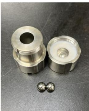
**Figure S2.** Stainless-steel jar (5 mL) and two stainless-steel balls (10 mm) used in this study.
