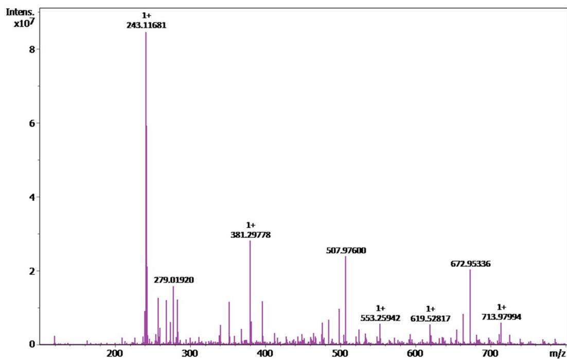
Figure S2. Accurate mass measurement of MTs/N<sub>3</sub>@AuNPs using LDI-FTICR MS.  $m/z$  243.1168 represented the triphenylmethyl cation released from MTs. Increasing the laser energy can obtain the signal of Au, but it will cause mass drift.
