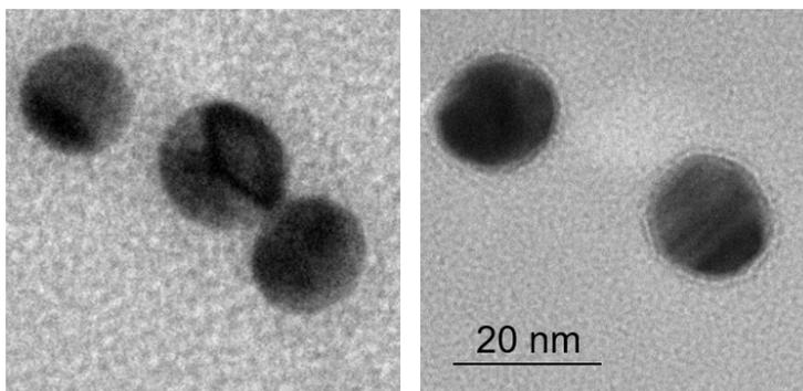
Figure S1. TEM images of bare AuNPs (left) and MTs/N<sub>3</sub>@AuNPs (right).
