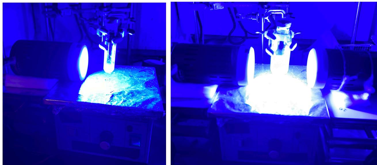
**Figure S1.** Pictures for reaction set-up with Kessil KSPR160L (456 nm, 40 W). The distance between the light source and reaction vessel was 2.0 cm. left: with one light source, right: with two light sources.
