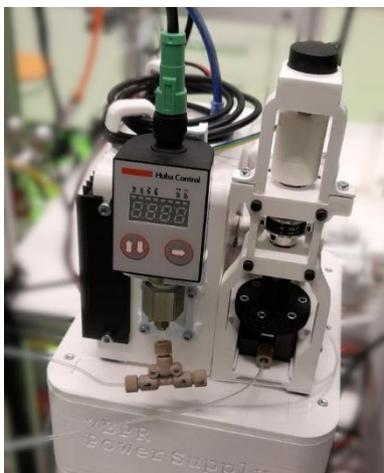
Figure S30 Variable back pressure regulator module with dedicated power supply.
