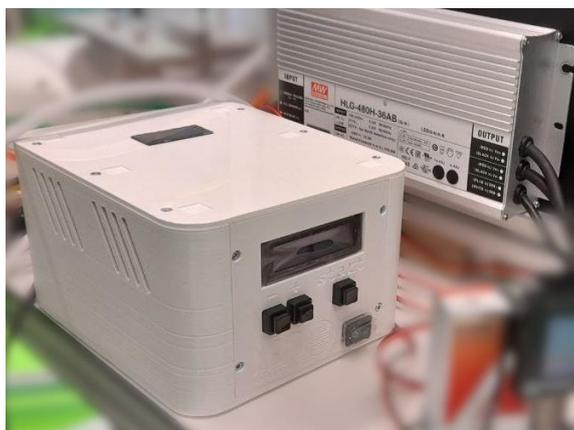
Figure S25 Light intensity control module (left) and LED power supply (right).
