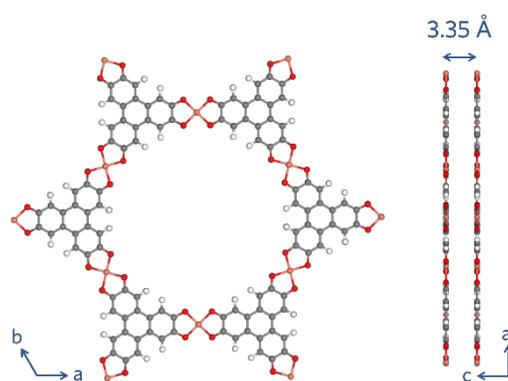
**Fig. S7** Structural models of Cu-HHTP viewed along c-axis (left) and b-axis (right).
