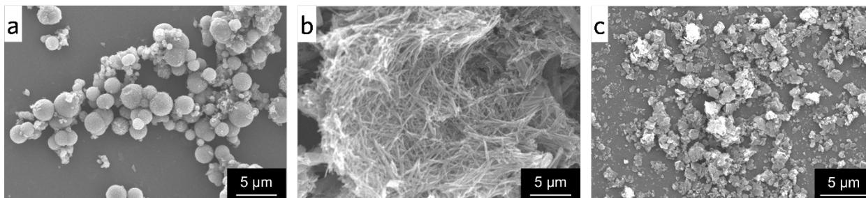
**Fig. S4** SEM image of (a) 0D, (b) 1D, and (c) 2D Cu-HHTP at a lower magnification.
