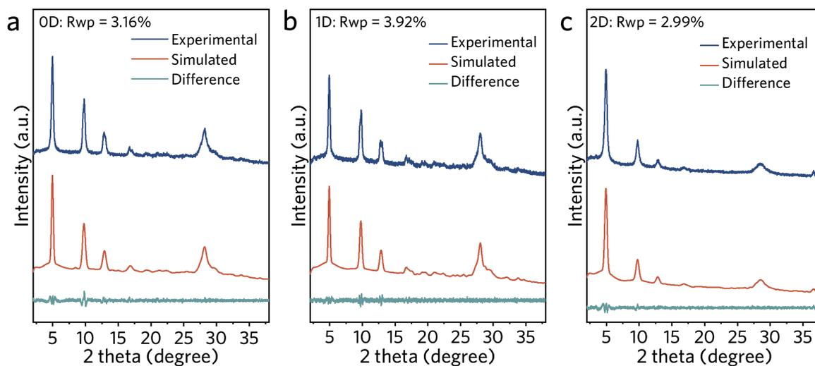
**Fig. S6** Experimental PXRd patterns of (a) 0D, (b) 1D, and (c) 2D Cu-HHTPs against the simulated eclipsed Cu-HHTP.
