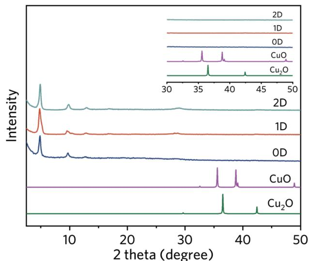
**Fig. S5** PXRd patterns of 0D, 1D, and 2D Cu-HHTP and possible impurities (Cu<sub>2</sub>O and CuO). Inset: A zoomed-in view in the range of 30° - 50°.
