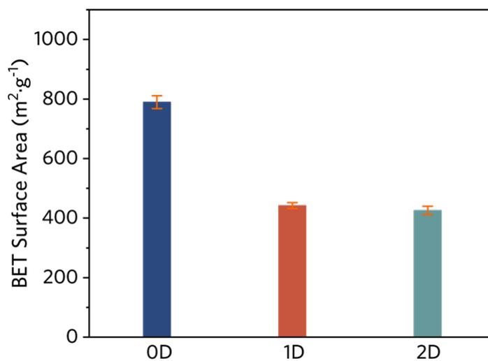
**Fig. S10** BET surface area of 0D, 1D, and 2D Cu-HHTP.
