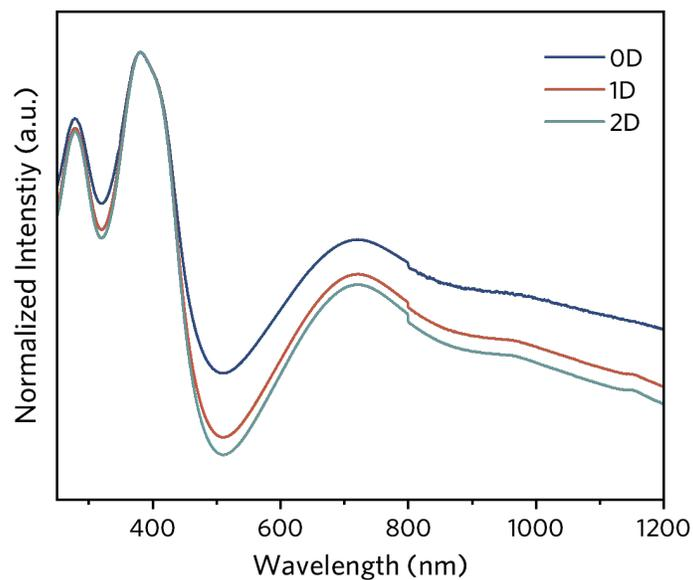
**Fig. S16** UV–vis-NIR absorption spectra of 1D, 2D, and 0D Cu-HHTP.
