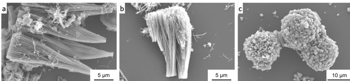
**Fig. S12** SEM images for the fragments of the 0D by microwave method with temperature-controlled ultrasonication.
