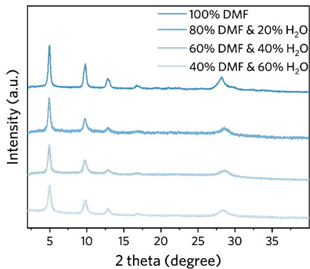
**Fig. S3** PXR D of 0D Cu-HHTP synthesized with different solvent ( $x\%$  DMF and  $(100-x)\%$  H<sub>2</sub>O).
