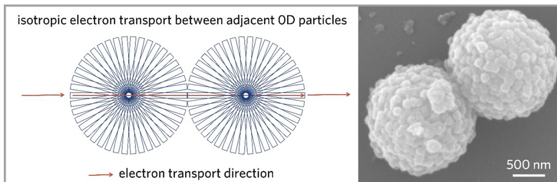
**Fig. S13** Schematic of hypothetical isotropic electron transport between adjacent 0D Cu-HHTP particles and the respective SEM image.
