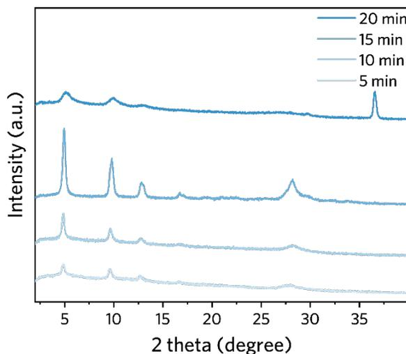
**Fig. S2** PXR D of 0D Cu-HHTP synthesized with different reaction time.
