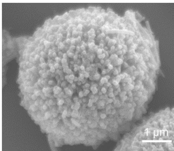
**Fig. S9** SEM image of 0D sphere Cu-HHTP, showing 0D crystals composed of smaller 1D rods.
