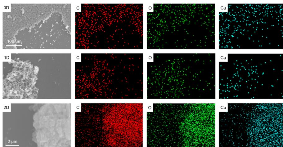
**Fig. S8** SEM-EDS elemental mapping images of 0D, 1D, and 2D Cu-HHTP.
