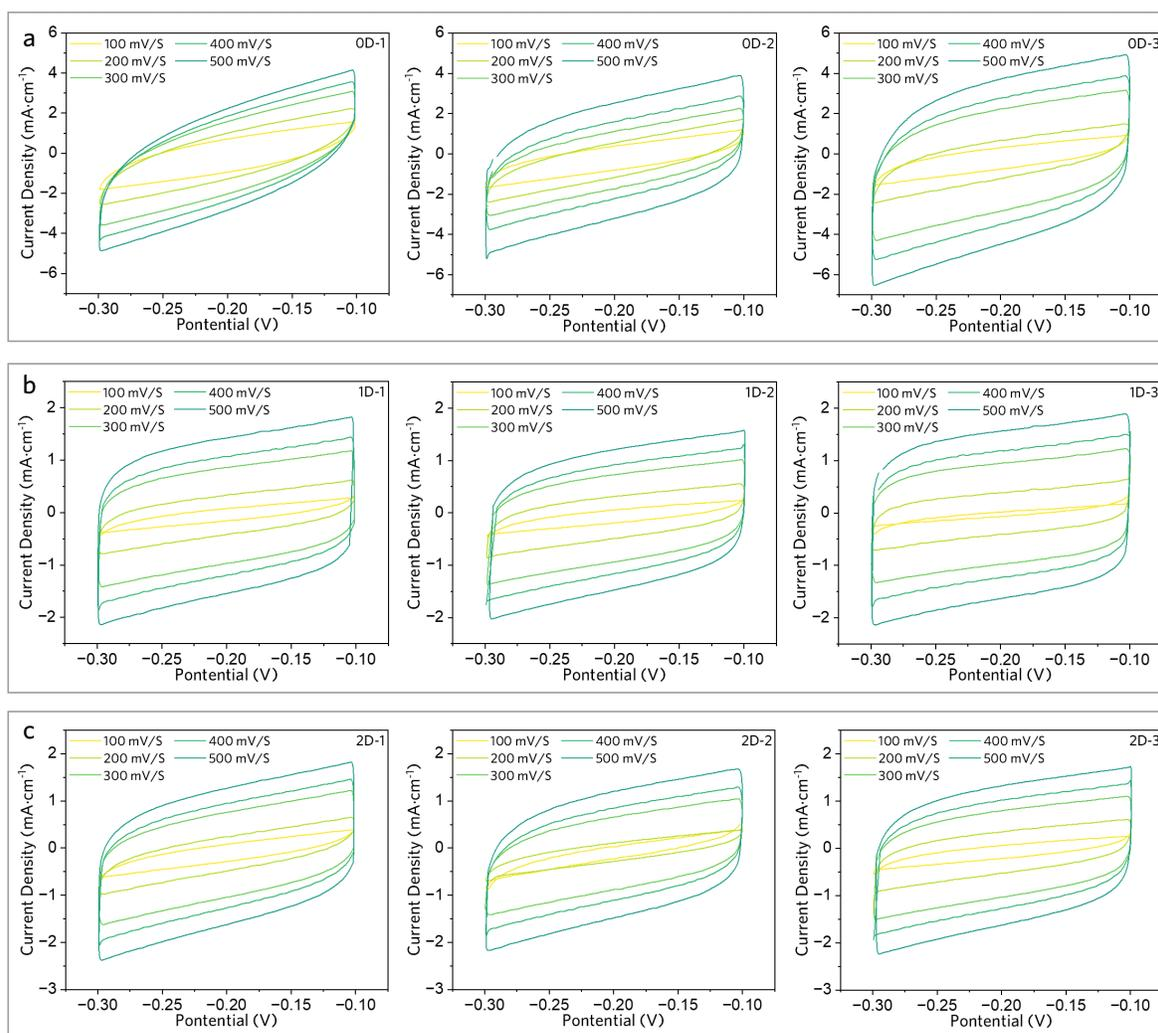
**Fig. S15** ECSA analysis of (a) 0D, (b) 1D, and (c) 2D Cu-HHTP based on double layer capacitance with scan rates ranging from 100 to 500 mV s<sup>-1</sup>, showing triplicate experiments for each sample.
