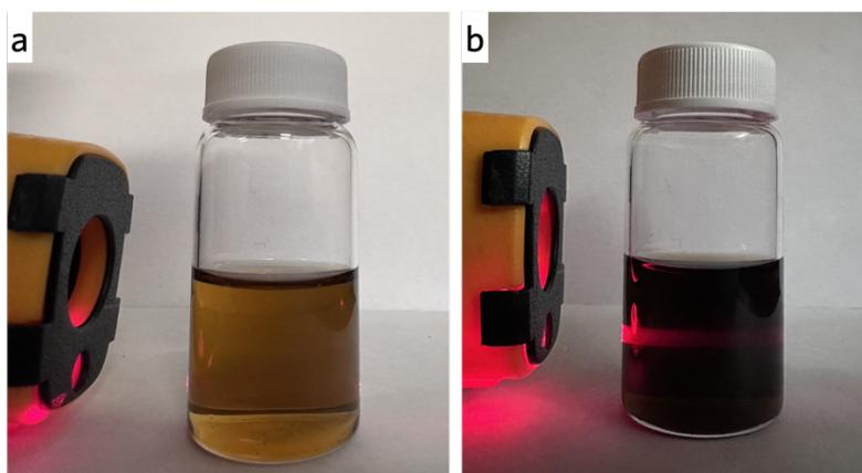
**Fig. S11** Tyndall effect in solution (a) before and (b) after temperature-controlled ultrasonication.
