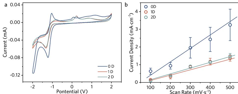
**Fig. S14** (a) Cyclic voltammetry curves of 0D, 1D, and 2D Cu-HHTP. (b) Plots of changing current density as a function of scan rate for 0D, 1D, and 2D Cu-HHTP.
