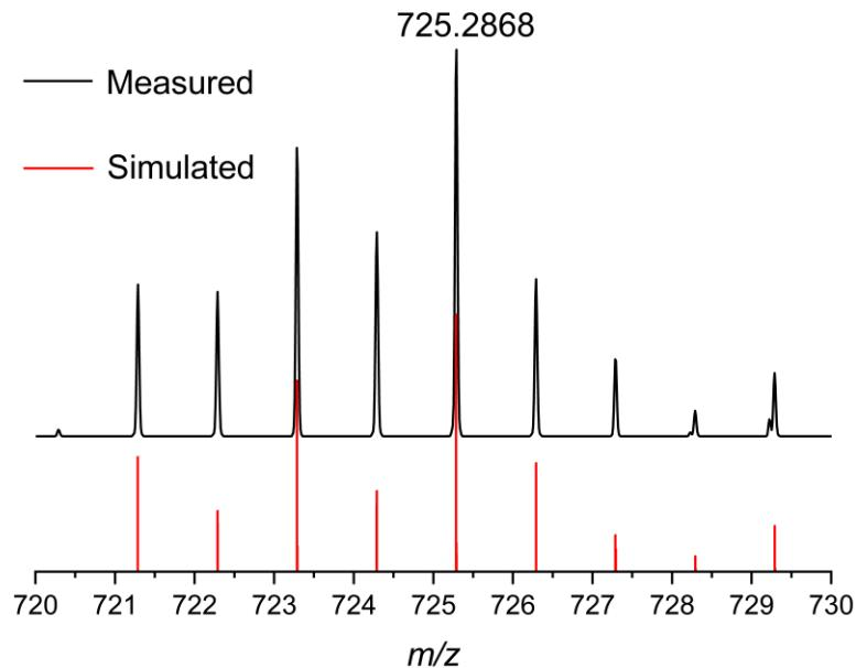
**Figure S19.** LIFDI-MS spectrum (detail view) of  $[3]^+$  in  $[3][\text{BArF}]$  (measured spectrum: top; simulated spectrum: bottom).
