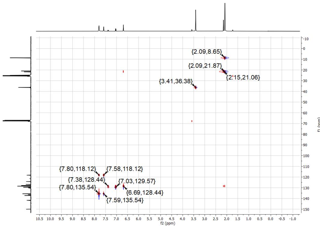
**Figure S3.**  $^1\text{H}/^{13}\text{C}$  NMR HSQC spectrum of **[2][BArF]** in  $\text{THF-d}_8$  at 298 K.
