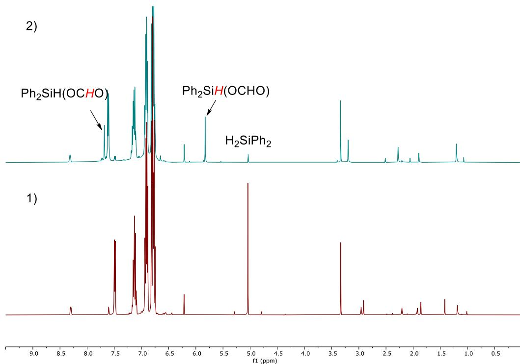
**Figure S43.** Stacked  $^1\text{H}$  NMR spectra of hydrosilylation of  $\text{CO}_2$  with  $\text{H}_2\text{SiPh}_2$  by [3][BArF]:
