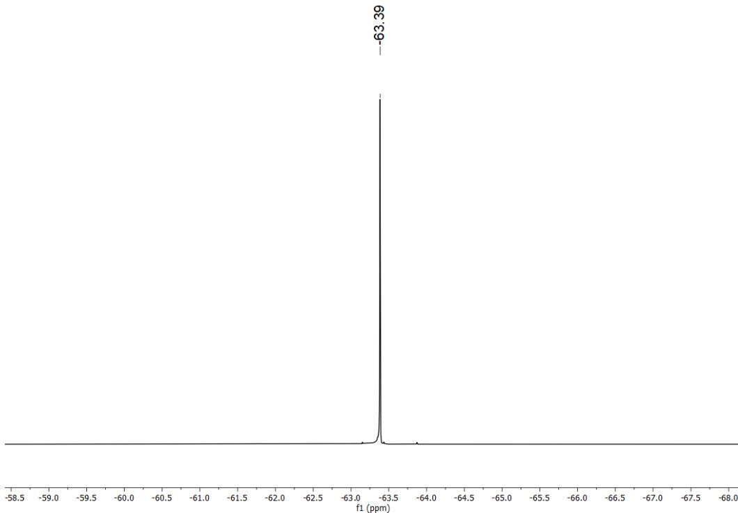
**Figure S18.**  $^{19}\text{F}\{^1\text{H}\}$  NMR spectrum of **[3][BArF]** in THF-d<sub>8</sub> at 298 K.
