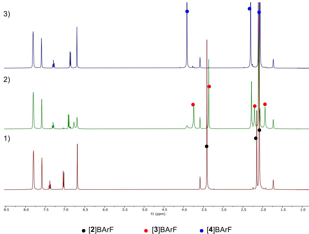
**Figure S21.** Stacked  $^1\text{H}$  NMR spectra of the reaction of  $[2]\text{[BArF]}$  with  $\text{CO}_2$  (1 bar): 1)  $[2]\text{[BArF]}$ ; 2)  $[2]\text{[BArF]} + \text{CO}_2$ , RT 6 hours; 3)  $[2]\text{[BArF]} + \text{CO}_2$ , RT 21 hours.
