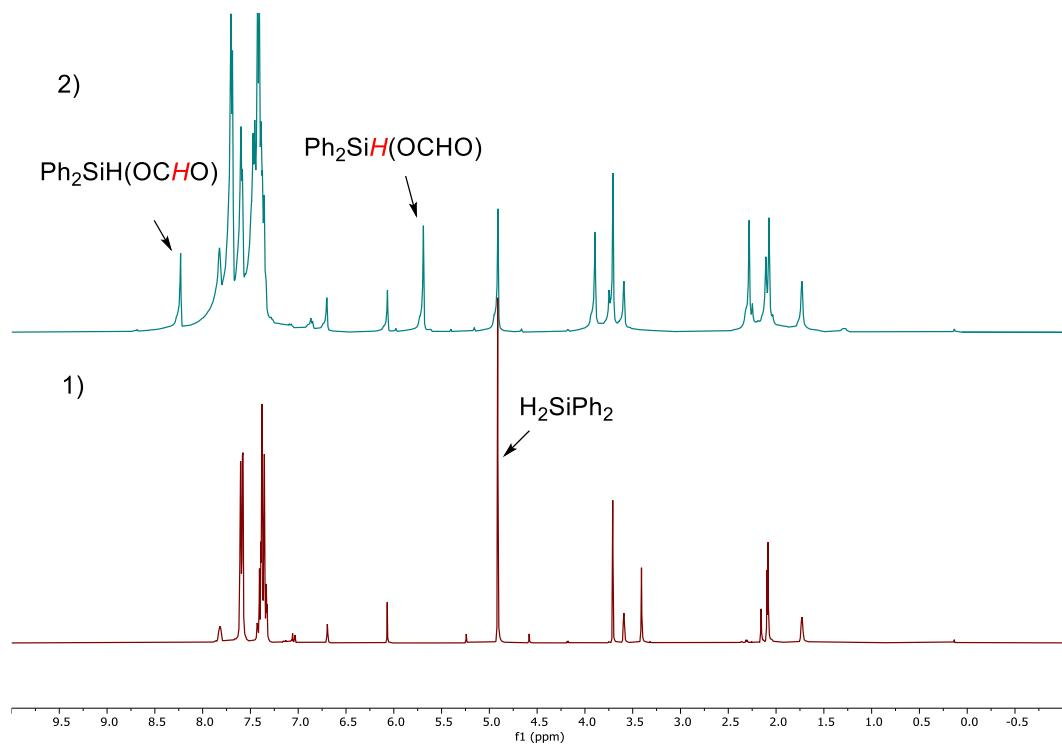
**Figure S37.** Stacked  $^1\text{H}$  NMR spectra of hydrosilylation of  $\text{CO}_2$  with  $\text{H}_2\text{SiPh}_2$  by [2][BArF] in THF-d<sub>8</sub>: 1) [2][BArF] (5 mol%) +  $\text{H}_2\text{SiPh}_2$ ; 2) [2][BArF] (5 mol%) +  $\text{H}_2\text{SiPh}_2$  +  $\text{CO}_2$ , RT 25 hours.
