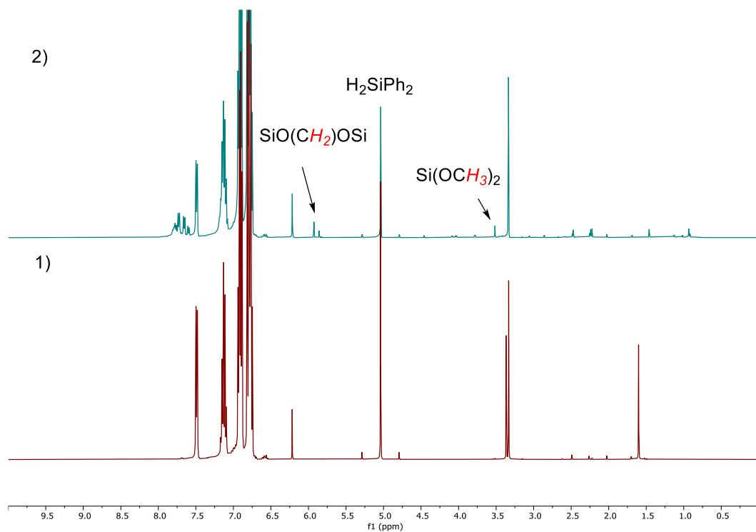
**Figure S45.** Stacked  $^1\text{H}$  NMR spectra of hydrosilylation of  $\text{CO}_2$  with  $\text{H}_2\text{SiPh}_2$  by  $\text{IMe}_4$ : 1)  $\text{IMe}_4$  (10 mol%) +  $\text{H}_2\text{SiPh}_2$ ; 2)  $\text{IMe}_4$  +  $\text{H}_2\text{SiPh}_2$  +  $\text{CO}_2$ , after 25 hours.
