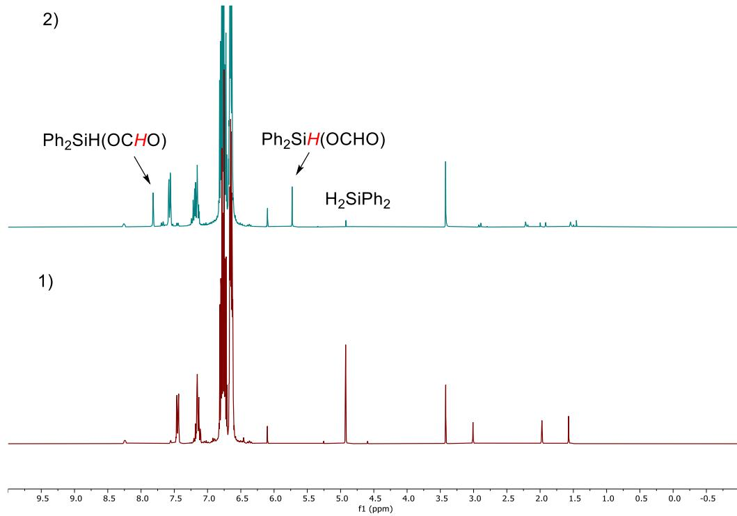
**Figure S39.** Stacked <sup>1</sup>H NMR spectra of hydrosilylation of CO<sub>2</sub> with H<sub>2</sub>SiPh<sub>2</sub> by [2][BArF] in C<sub>6</sub>D<sub>6</sub>/C<sub>6</sub>H<sub>4</sub>F<sub>2</sub> (1:1): 1) [2][BArF] (5 mol%) + H<sub>2</sub>SiPh<sub>2</sub>; 2) [2][BArF] (5 mol%) + H<sub>2</sub>SiPh<sub>2</sub> + CO<sub>2</sub>, RT 25 hours.
