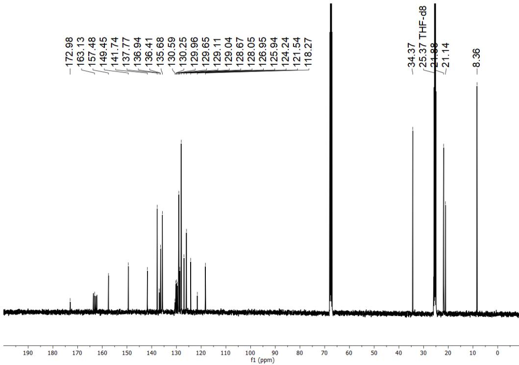
**Figure S22.**  $^{13}\text{C}\{\text{H}\}$  NMR spectrum of [4][BArF] in THF-d<sub>8</sub> at 298 K.
