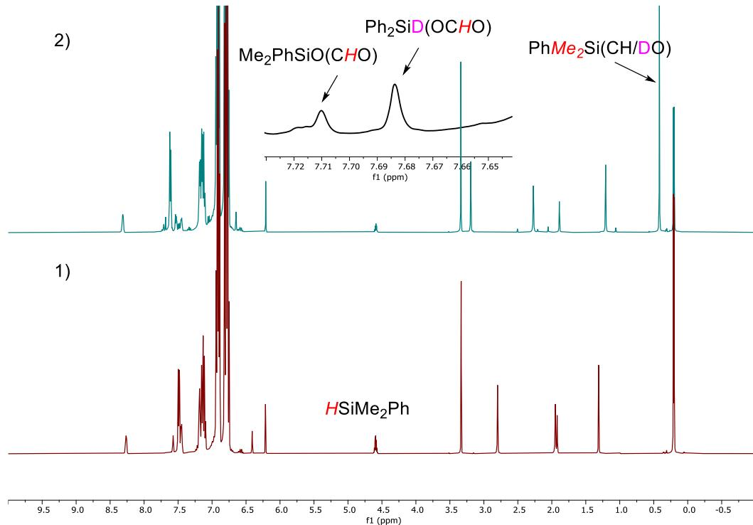
**Figure S54.** Stacked  $^1\text{H}$  NMR spectra of hydrosilylation of  $\text{CO}_2$  with  $\text{D}_2\text{SiPh}_2/\text{HSiMe}_2\text{Ph}$  by [2][BArF]: 1) [2][BArF] (5 mol%) +  $\text{D}_2\text{SiPh}_2$  +  $\text{HSiMe}_2\text{Ph}$ ; 2) [2][BArF] (5 mol%) +  $\text{D}_2\text{SiPh}_2$  +  $\text{HSiMe}_2\text{Ph}$  +  $\text{CO}_2$ , RT 25 hours.
