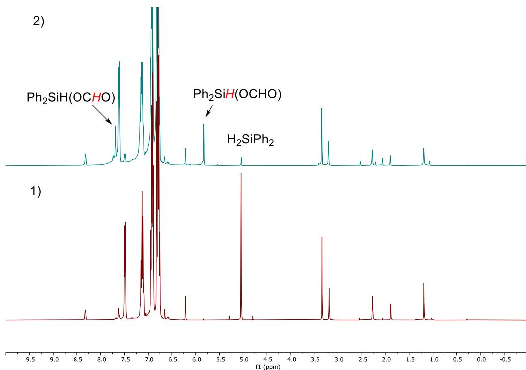
**Figure S44.** Stacked  $^1\text{H}$  NMR spectra of hydrosilylation of  $\text{CO}_2$  with  $\text{H}_2\text{SiPh}_2$  by [4][BArF]:
