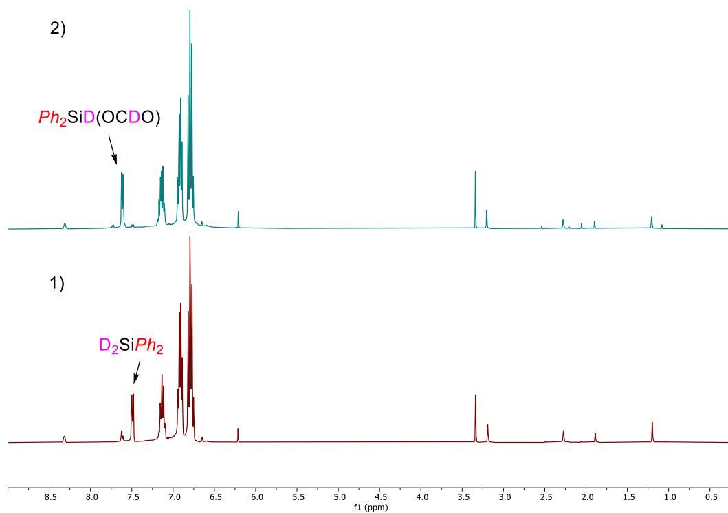
**Figure S51.** Stacked  $^1\text{H}$  NMR spectra of hydrosilylation of  $\text{CO}_2$  with  $\text{D}_2\text{SiPh}_2$  by  $[4]\text{[BArF]}$ : 1)  $[4]\text{[BArF]}$  (5 mol%) +  $\text{D}_2\text{SiPh}_2$ ; 2)  $[4]\text{[BArF]}$  (5 mol%) +  $\text{H}_2\text{SiPh}_2$  +  $\text{CO}_2$ , RT 25 hours.
