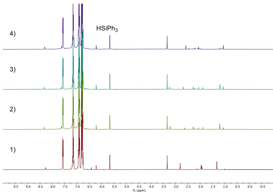
**Figure S50.** Stacked  $^1\text{H}$  NMR spectra of hydrosilylation of  $\text{CO}_2$  with  $\text{HSiPh}_3$  by **[2][BArF]**: 1) **[2][BArF]** (5 mol%) +  $\text{HSiPh}_3$ ; 2) **[2][BArF]** (5 mol%) +  $\text{HSiPh}_3$  +  $\text{CO}_2$ , RT 17 hours + 60 °C 18 hours + 80 °C 18 hours.
