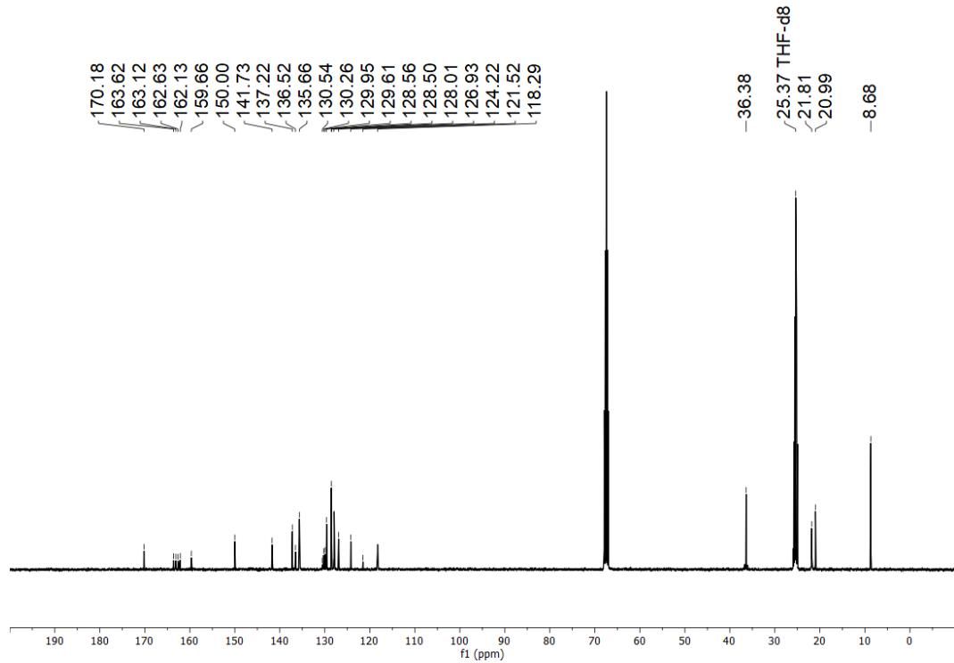
**Figure S2.** <sup>13</sup>C{<sup>1</sup>H} NMR spectrum of [2][BArF] in THF-d<sub>8</sub> at 298 K.
