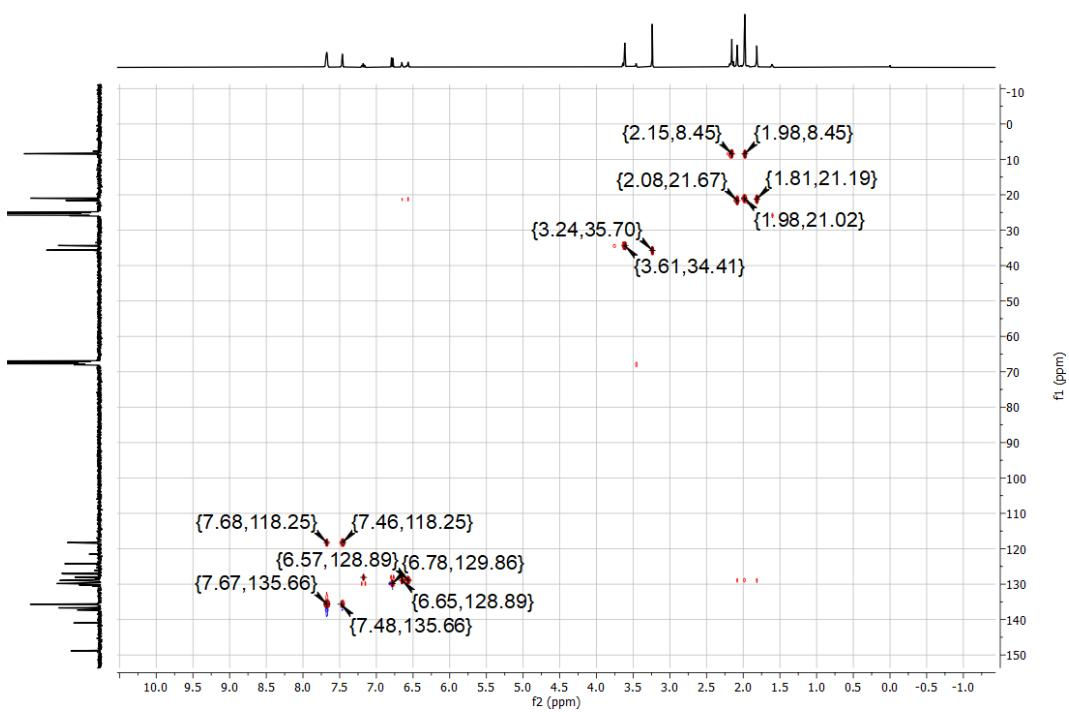
**Figure S15.**  $^1\text{H}/^{13}\text{C}$  NMR HSQC spectrum of  $[\mathbf{3}][\text{BArF}]$  in  $\text{THF-d}_8$  at 298 K.
