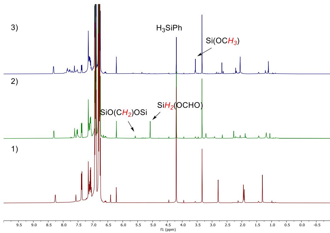
**Figure S48.** Stacked  $^1\text{H}$  NMR spectra of hydrosilylation of  $\text{CO}_2$  with  $\text{H}_3\text{SiPh}$  by  $[\mathbf{2}][\text{BArF}]$ : 1)  $[\mathbf{2}][\text{BArF}]$  (5 mol%) +  $\text{H}_3\text{SiPh}$ ; 2)  $[\mathbf{2}][\text{BArF}]$  (5 mol%) +  $\text{H}_3\text{SiPh}$  +  $\text{CO}_2$ , RT 2 hours;  $[\mathbf{2}][\text{BArF}]$  (5 mol%) +  $\text{H}_3\text{SiPh}$  +  $\text{CO}_2$ , RT 12 hours.
