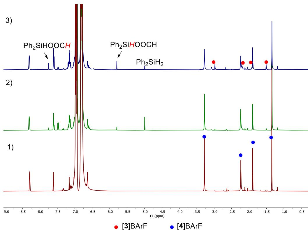
**Figure S31.** Stack the  $^1\text{H}$  NMR spectra showing [4][BArF] reaction with  $\text{Ph}_2\text{SiH}_2$ : 1) the formation of [4][BArF]; 2) [4][BArF] +  $\text{H}_2\text{SiPh}_2$ , RT 1 hour; 3) [4][BArF] +  $\text{H}_2\text{SiPh}_2$ , RT 5 hours.
