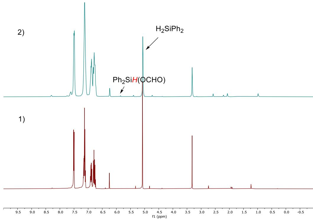
**Figure S33.** Stacked  $^1\text{H}$  NMR spectra of hydrosilylation of  $\text{CO}_2$  with  $\text{H}_2\text{SiPh}_2$  by [2][BArF] (1 mol%) in  $\text{C}_6\text{D}_6/\text{C}_6\text{H}_5\text{F}$  (4:1): 1) [2][BArF] (1 mol%) +  $\text{H}_2\text{SiPh}_2$ ; 2) [2][BArF] (1 mol%) +  $\text{H}_2\text{SiPh}_2$  +  $\text{CO}_2$ , RT 25 hours.
