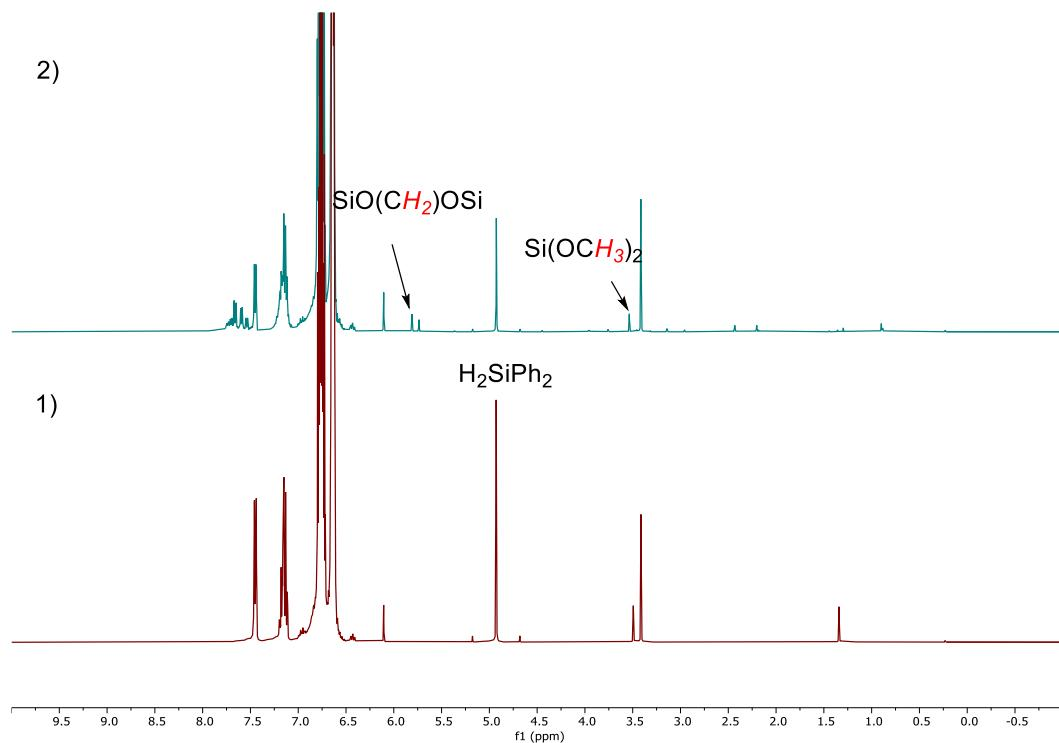
**Figure S46.** Stacked  $^1\text{H}$  NMR spectra of hydrosilylation of  $\text{CO}_2$  with  $\text{H}_2\text{SiPh}_2$  by  $\text{IMe}_4\text{-CO}_2$ : 1)  $\text{IMe}_4\text{-CO}_2$  (10 mol%) +  $\text{H}_2\text{SiPh}_2$ ; 2)  $\text{IMe}_4\text{-CO}_2$  +  $\text{H}_2\text{SiPh}_2$  +  $\text{CO}_2$ , RT 25 hours.
