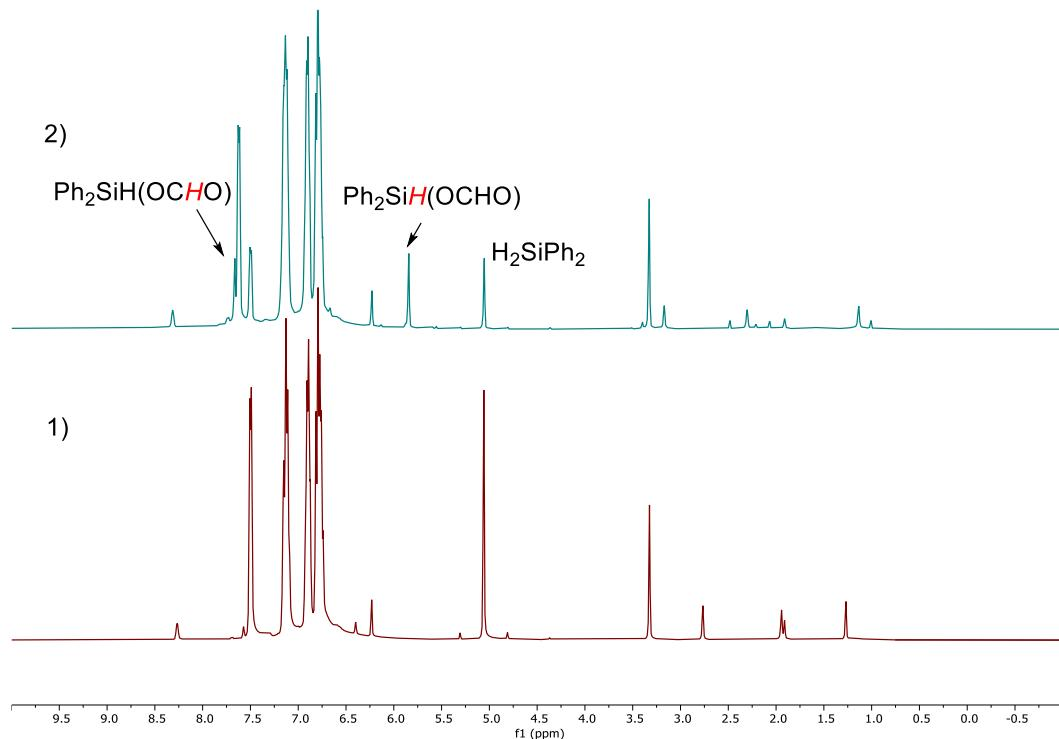
**Figure S34.** Stacked  $^1\text{H}$  NMR spectra of hydrosilylation of  $\text{CO}_2$  with  $\text{H}_2\text{SiPh}_2$  by  $[2]\text{[BArF]}$  (2.5 mol%) in  $\text{C}_6\text{D}_6/\text{C}_6\text{H}_5\text{F}$  (4:1): 1)  $[2]\text{[BArF]}$  (2.5 mol%) +  $\text{H}_2\text{SiPh}_2$ ; 2)  $[2]\text{[BArF]}$  (2.5 mol%) +  $\text{H}_2\text{SiPh}_2 + \text{CO}_2$ , RT 25 hours.
