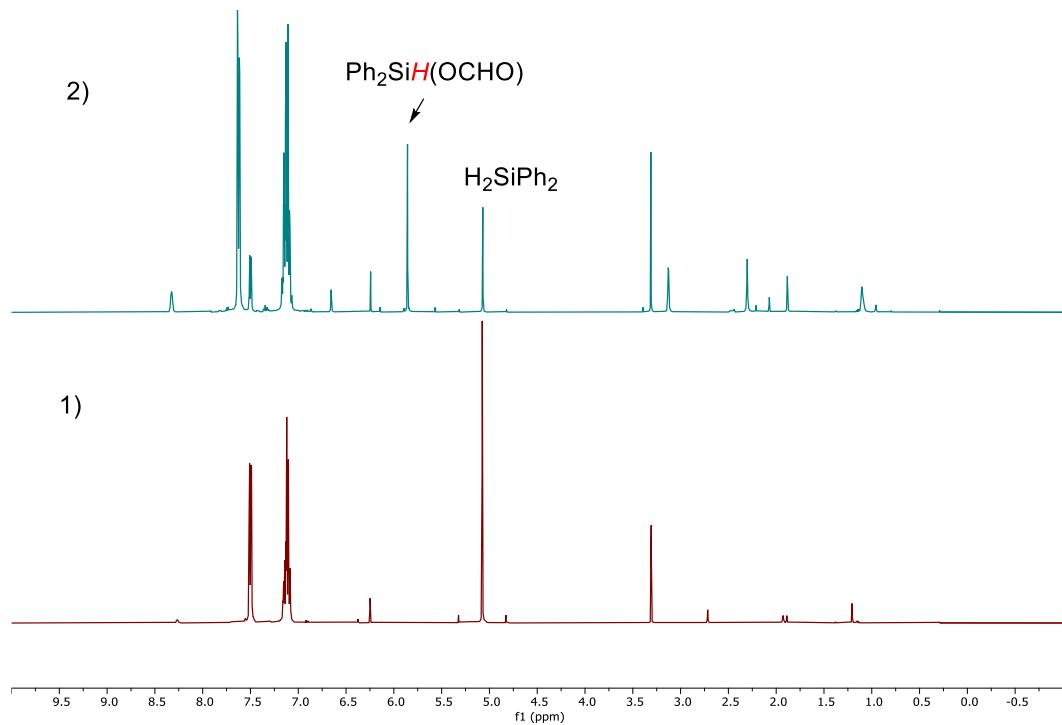
**Figure S36.** Stacked <sup>1</sup>H NMR spectra of hydrosilylation of CO<sub>2</sub> with H<sub>2</sub>SiPh<sub>2</sub> by **[2][BArF]** in C<sub>6</sub>D<sub>6</sub>: 1) **[2][BArF]** (5 mol%) + H<sub>2</sub>SiPh<sub>2</sub>; 2) **[2][BArF]** (5 mol%) + H<sub>2</sub>SiPh<sub>2</sub> + CO<sub>2</sub>, RT 25 hours.
