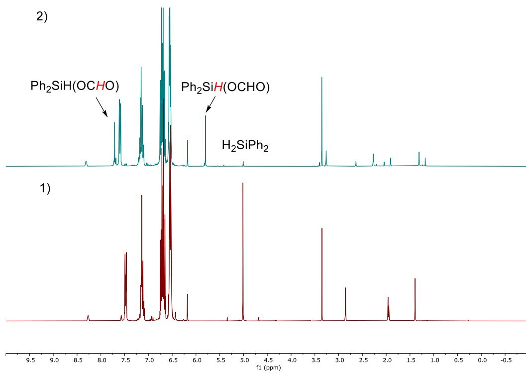
**Figure S38.** Stacked  $^1\text{H}$  NMR spectra of hydrosilylation of  $\text{CO}_2$  with  $\text{H}_2\text{SiPh}_2$  by [2][BArF] in  $\text{C}_6\text{D}_6/\text{C}_6\text{H}_4\text{F}_2$  (4:1): 1) [2][BArF] (5 mol%) +  $\text{H}_2\text{SiPh}_2$ ; 2) [2][BArF] (5 mol%) +  $\text{H}_2\text{SiPh}_2$  +  $\text{CO}_2$ , RT 25 hours.
