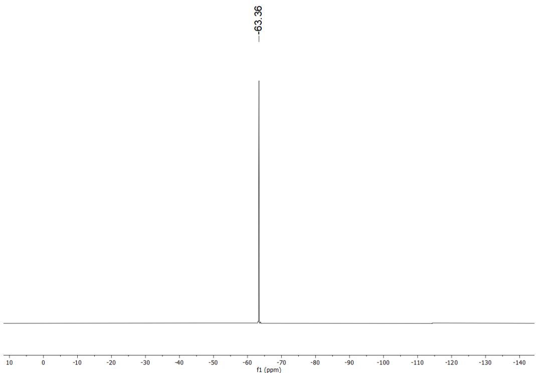
**Figure S26.**  $^{19}\text{F}\{\text{H}\}$  NMR spectrum of **[4][BArF]** in THF-d<sub>8</sub> at 298 K.
