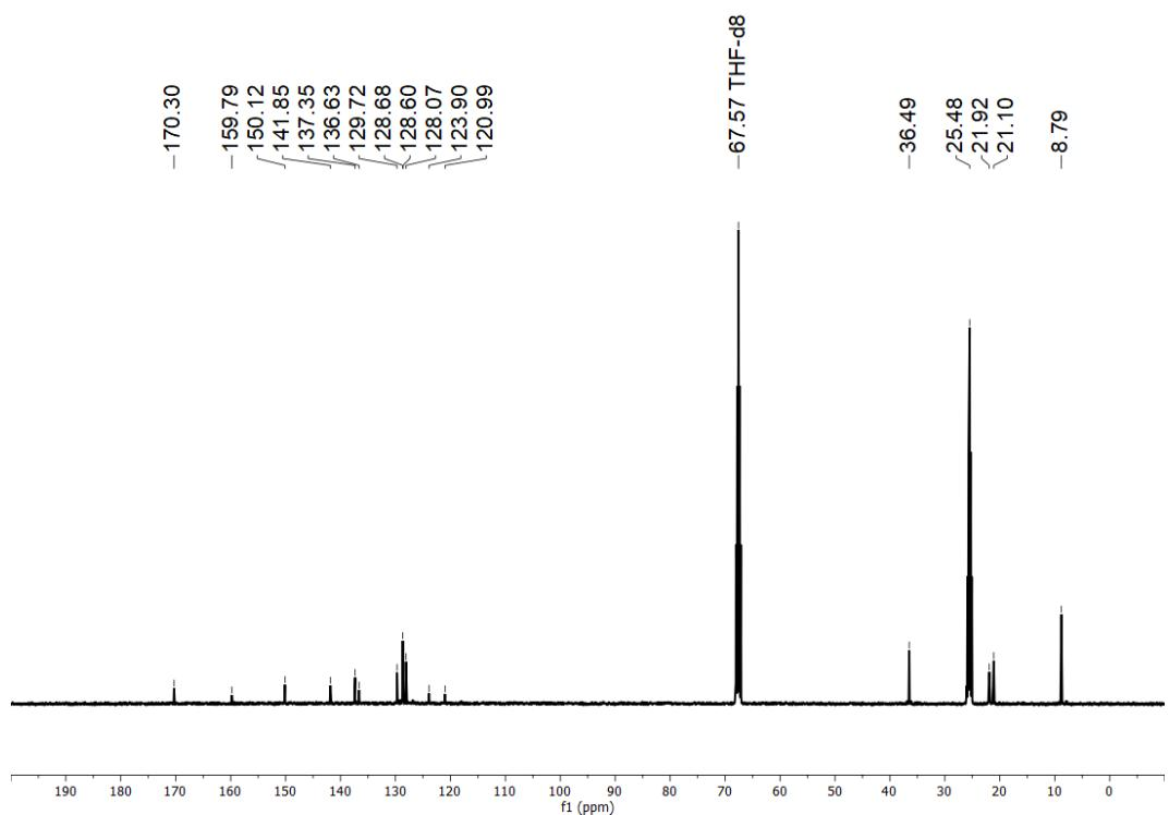
**Figure S9.**  $^{13}\text{C}\{{}^1\text{H}\}$  NMR spectrum of  $[2]\text{[Al(OC(CF}_3)_3)_4]$  in THF-d<sub>8</sub> at 298 K.
