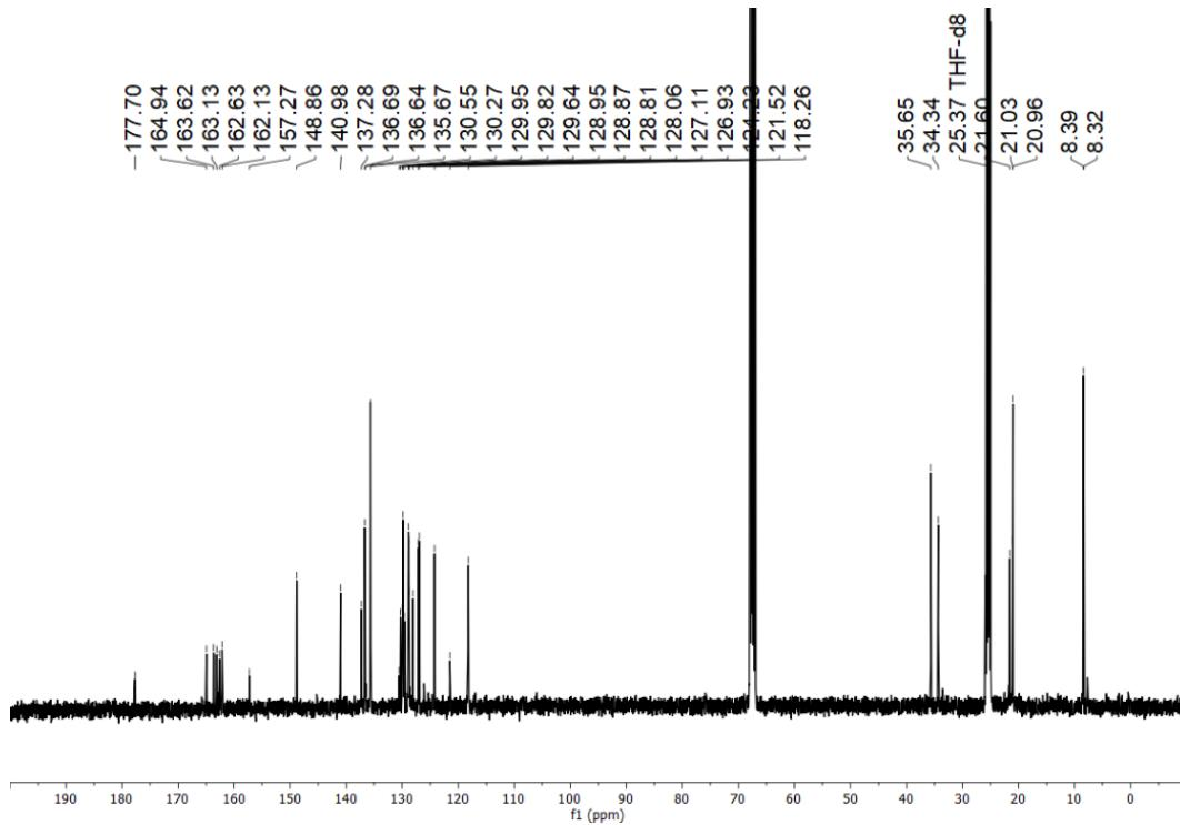
**Figure S14.**  $^{13}\text{C}\{^1\text{H}\}$  NMR spectrum of  $[3]\text{[BArF]}$  in  $\text{THF-d}_8$  at 298 K.
