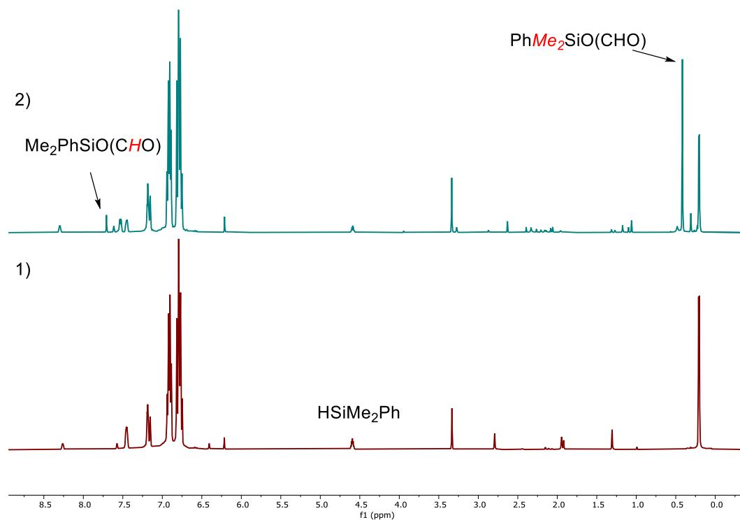
**Figure S47.** Stacked  $^1\text{H}$  NMR spectra of hydrosilylation of  $\text{CO}_2$  with  $\text{HSiMe}_2\text{Ph}$  by  $[\mathbf{2}][\text{BArF}]$ : 1)  $[\mathbf{2}][\text{BArF}]$  (5 mol%) +  $\text{HSiMe}_2\text{Ph}$ ; 2)  $[\mathbf{2}][\text{BArF}]$  (5 mol%) +  $\text{HSiMe}_2\text{Ph}$  +  $\text{CO}_2$ , RT 25 hours.
