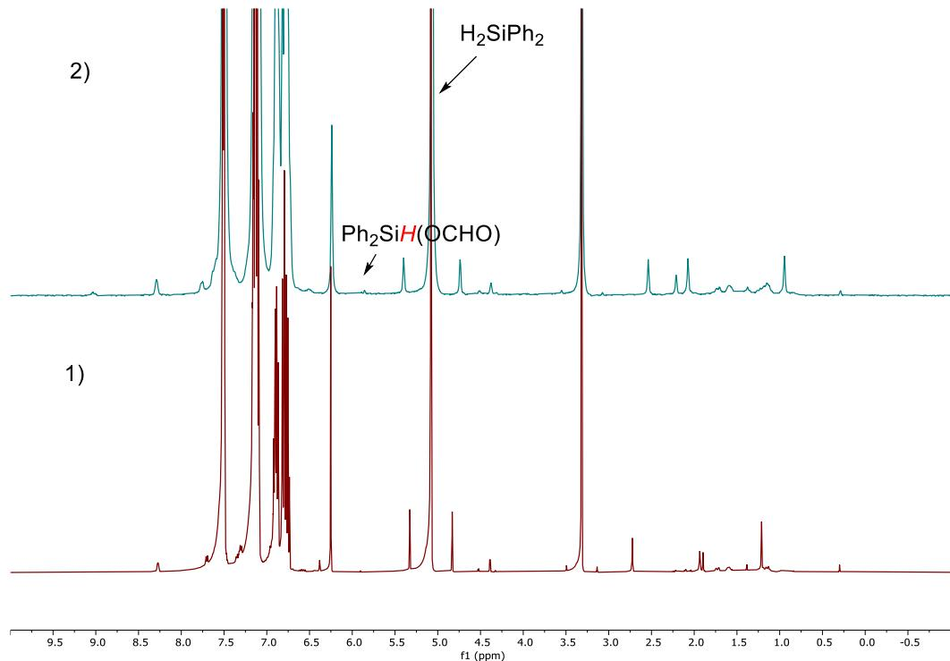
**Figure S32.** Stacked <sup>1</sup>H NMR spectra of hydrosilylation of  $\text{CO}_2$  with  $\text{H}_2\text{SiPh}_2$  by [2][BArF] (0.5 mol%) in  $\text{C}_6\text{D}_6/\text{C}_6\text{H}_5\text{F}$  (4:1): 1) [2][BArF] (0.5 mol%) +  $\text{H}_2\text{SiPh}_2$ ; 2) [2][BArF] (0.5 mol%) +  $\text{H}_2\text{SiPh}_2$  +  $\text{CO}_2$ , RT 25 hours.
