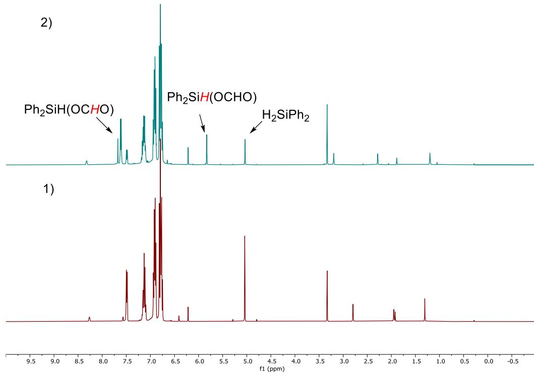
**Figure S42.** Stacked <sup>1</sup>H NMR spectra of hydrosilylation of CO<sub>2</sub> with H<sub>2</sub>SiPh<sub>2</sub> by [2][BArF] in C<sub>6</sub>D<sub>6</sub>/C<sub>6</sub>H<sub>5</sub>F (4:1) in the presence of Hg: 1) [2][BArF] (5 mol%) + H<sub>2</sub>SiPh<sub>2</sub>; 2) [2][BArF] (5 mol%) + H<sub>2</sub>SiPh<sub>2</sub> + CO<sub>2</sub>, RT 25 hours.
