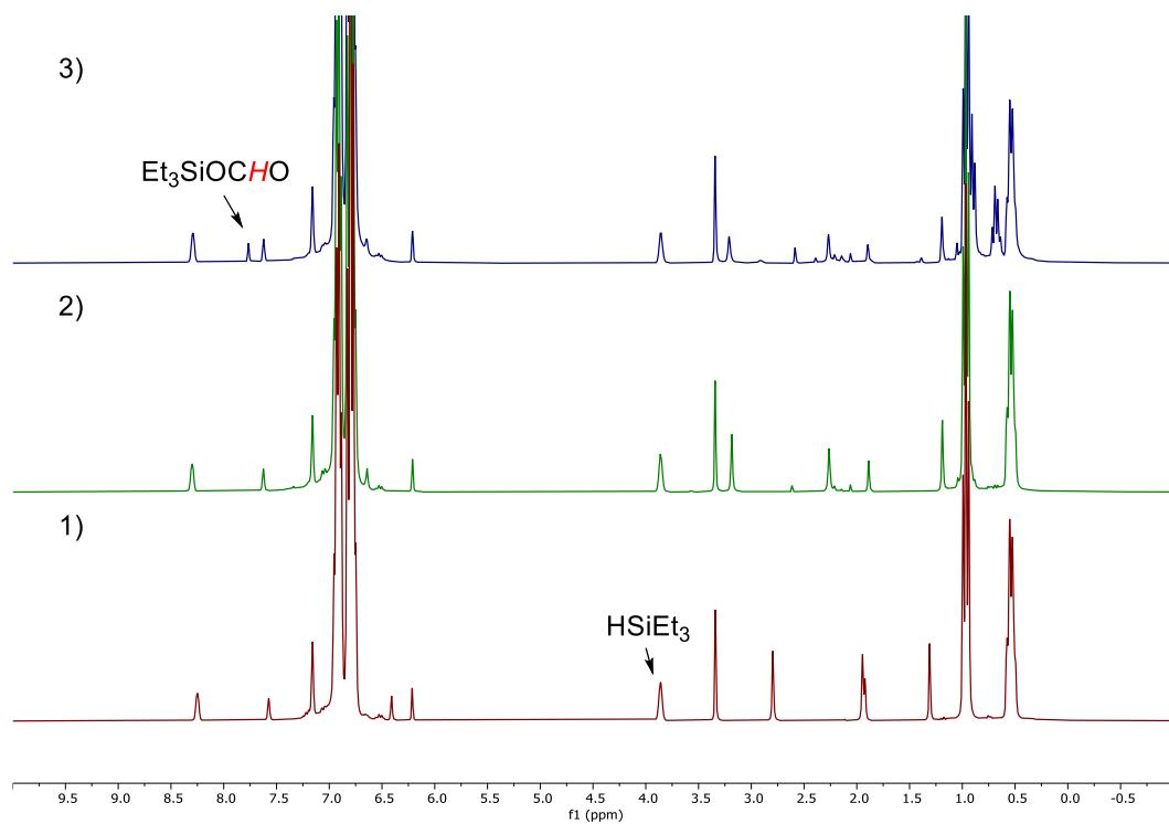
**Figure S49.** Stacked <sup>1</sup>H NMR spectra of hydrosilylation of CO<sub>2</sub> with HSiEt<sub>3</sub> by [2][BArF]: 1) [2][BArF] (5 mol%) + HSiEt<sub>3</sub>; 2) [2][BArF] (5 mol%) + HSiEt<sub>3</sub> + CO<sub>2</sub>, RT 21 hours; [2][BArF] (5 mol%) + HSiEt<sub>3</sub> + CO<sub>2</sub>, RT 21 hours + 60 °C 25 hours.
