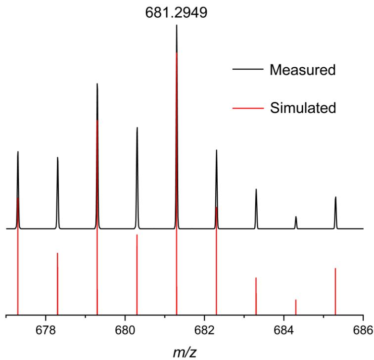
**Figure S12.** LIFDI-MS spectrum (detail view) of  $[2]^+$  in  $[2][\text{Al}(\text{OC}(\text{CF}_3)_3)_4]$  (measured spectrum: top; simulated spectrum: bottom).
