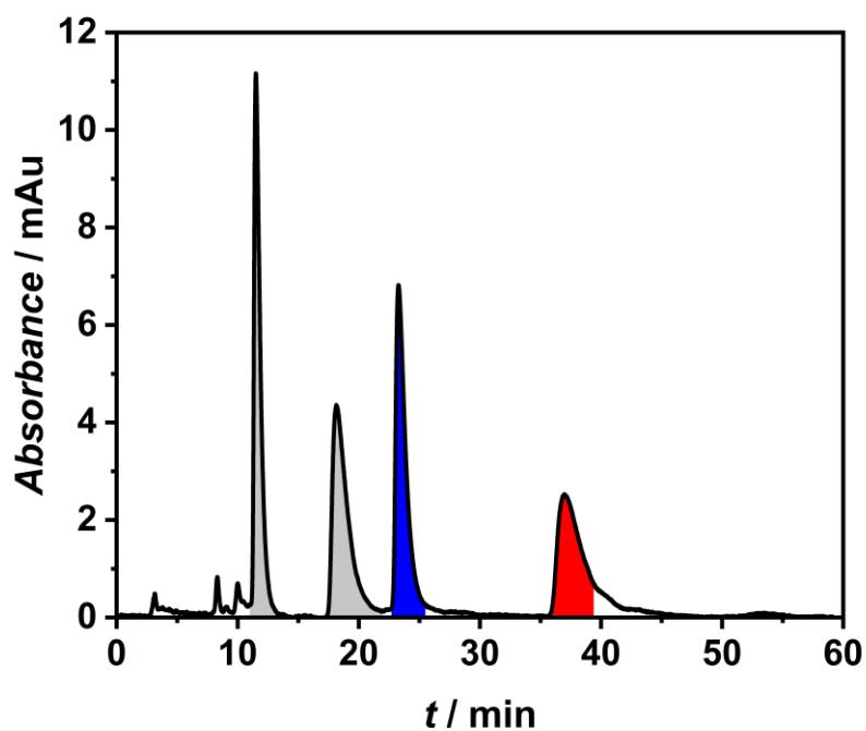
**Figure S19.** HPLC chromatogram of **2**. A racemate was injected and recycled (grey) until peak separation. Enantiomer 1 (blue) and enantiomer 2 (red) were collected in the 2nd cycle and correspond to ( $S_P$ )- and ( $R_P$ )-enantiomers, respectively.
