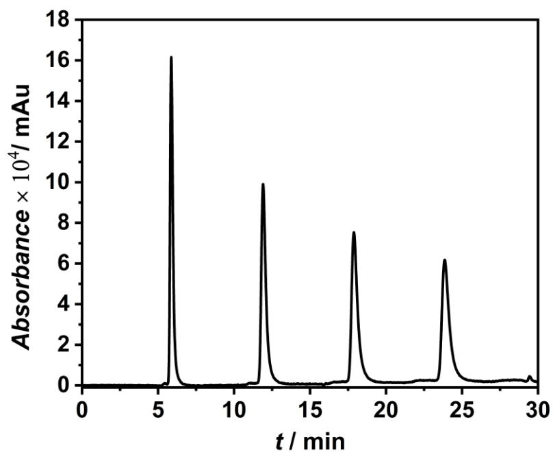
**Figure S58.** Analytical HPLC chromatogram of enantiomer 1 reinjection for **3** on Phenomenex IC column (flow rate: 3 ml/min, 100% Chloroform) which corresponds to (*R<sub>P</sub>*)-enantiomer.
