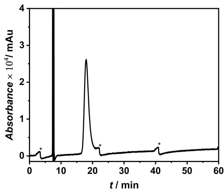
**Figure S60.** Analytical HPLC chromatogram of enantiomer 1 reinjection for **3** on the Chiralpak IG column (4.6x250mm, Flow rate: 1 ml/ min, toluene/TBME/*n*-heptane, v/v, 1:7:2) which corresponds to (*R<sub>P</sub>*)-enantiomer. \* = sudden change in the baseline signal.
