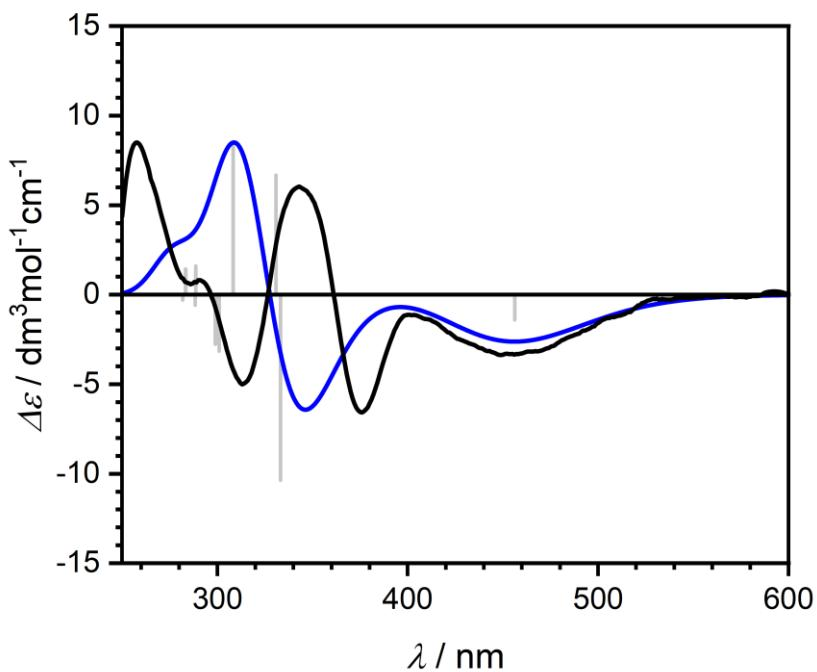
**Figure S31.** Experimental (black) and calculated (blue) CD spectra of ( $R_P$ )-**2** with excitation transitions (grey lines).
