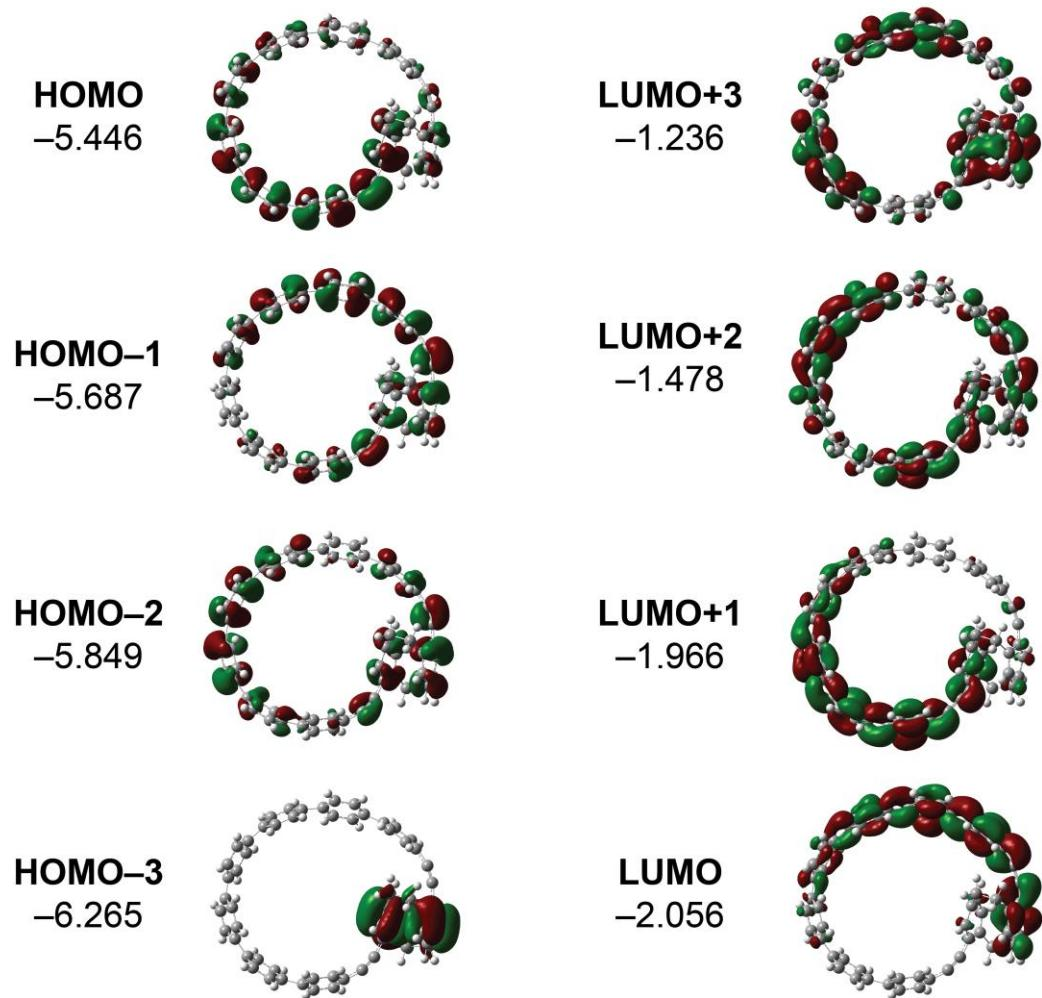
**Figure S51.** Frontier molecular orbitals of **1'** with energies in eV.
