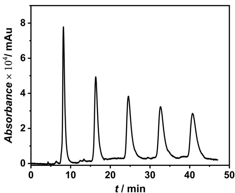
**Figure S59.** Analytical HPLC chromatogram of enantiomer 2 reinjection for **3** on Phenomenex IC column (flow rate: 3 ml/min, 100% Chloroform) which corresponds to (*S<sub>P</sub>*)-enantiomer.
