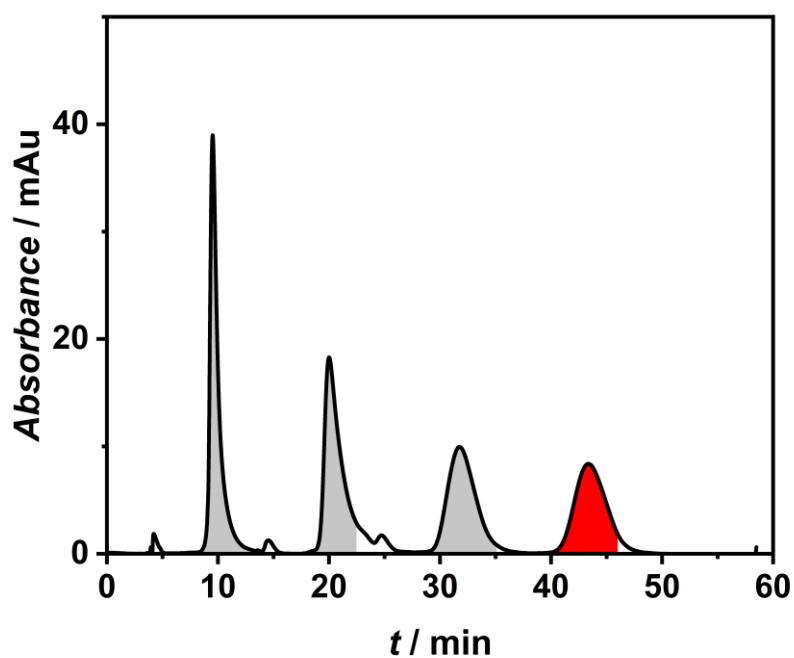
**Figure S21.** HPLC chromatogram of enantiomer 1 reinjection for **3**. The peak was recycled (grey) for 3 times before collection (red) and corresponds to (*R<sub>P</sub>*)-enantiomer. The sample was then reinjected to analytical HPLC to confirm its purity.
