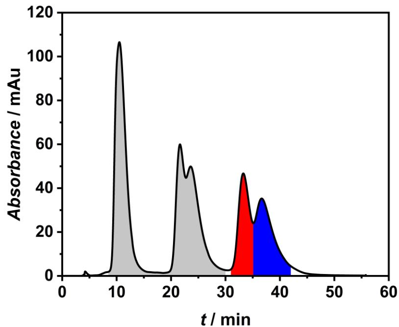
**Figure S20.** HPLC chromatogram of **3**. A racemate was injected and recycled (grey) until peak separation. Enantiomer 1 (red) and enantiomer 2 (blue) were collected in the 3rd cycle and correspond to ( $R_P$ )- and ( $S_P$ )-enantiomers, respectively.
