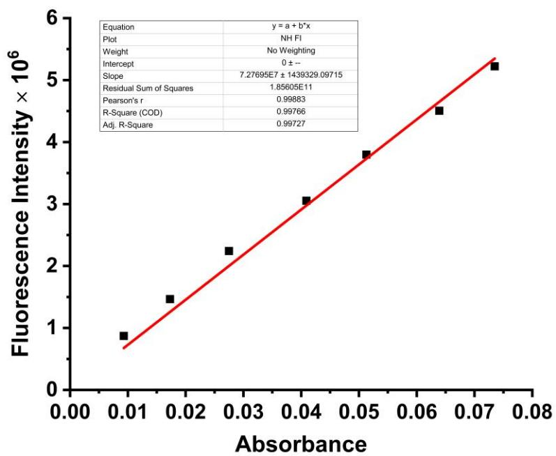
**Figure S17.** Integrated fluorescence intensity vs absorbance for **2**.
