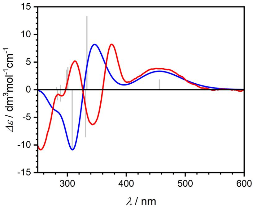
**Figure S32.** Experimental (red) and calculated (blue) CD spectra of ( $S_P$ )-**2** with excitation transitions (grey lines).
