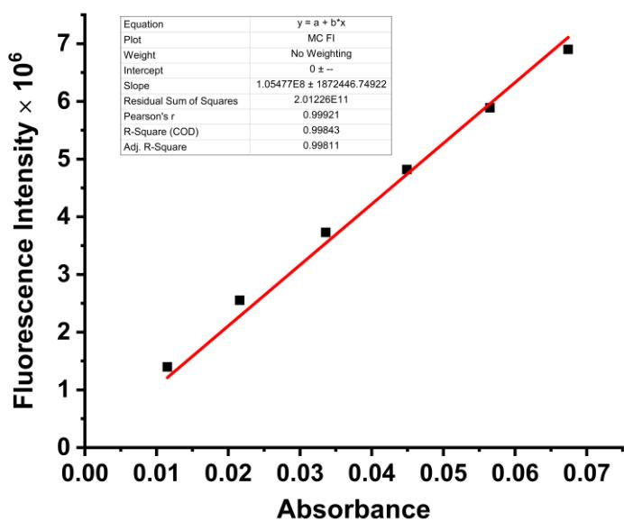
**Figure S18.** Integrated fluorescence intensity vs absorbance for **3**.
