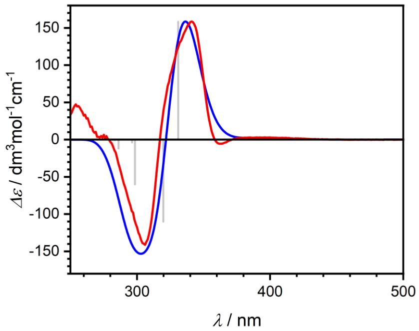
**Figure S34.** Experimental (red) and calculated (blue) CD spectra of ( $S_P$ )-3 with excitation transitions (grey lines).
