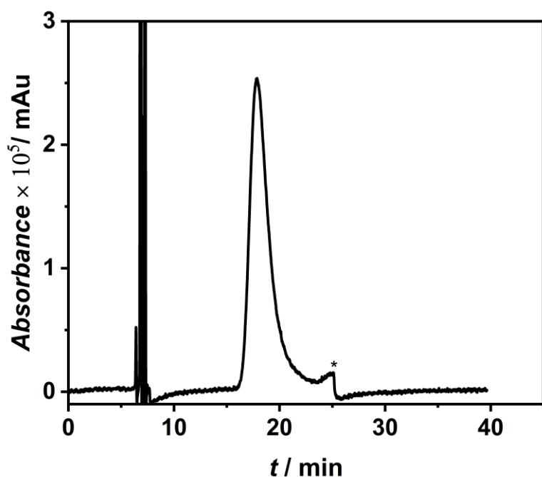
**Figure S61.** Analytical HPLC chromatogram of enantiomer 2 reinjection for **3** on the Chiralpak IG column (4.6x250mm, Flow rate: 1 ml/ min, toluene/TBME/*n*-heptane, v/v, 1:7:2) which corresponds to (*S*<sub>P</sub>)-enantiomer. \* = sudden change in the baseline signal.
