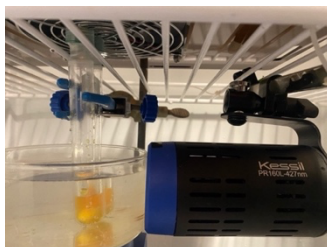
Figure S7. Reaction apparatus of hydroxytrifluoromethylation irradiated under 427 nm. (LED light source: Kessil LEDs 427 nm)
