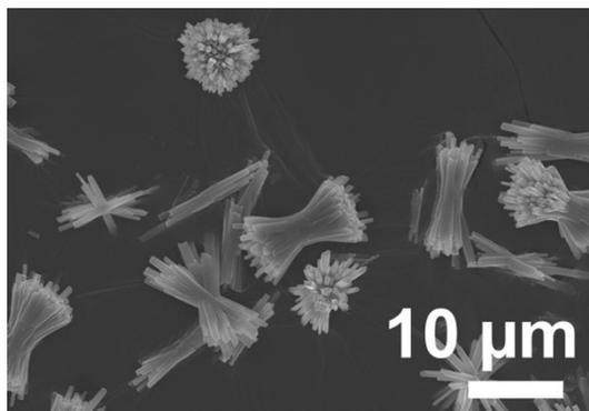
**Figure S2.** SEM image of  $\text{La}(\text{BTC})(\text{H}_2\text{O})_6$ .
