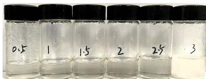
**Fig. S1** Optical images of SN-LiTFSI with different molar ratios of SN and LiTFSI at room temperature.
