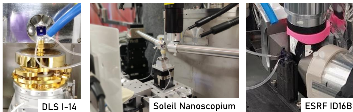
Figure S8. Custom microfluidic device for liquid cell measurements installed at Diamond Light Source I14, Soleil Synchrotron Nanoscopia and ESRF ID16B.
