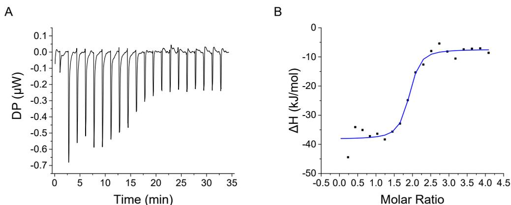
**Fig. S1** ITC measurement (A) and binding isotherm fitted by one-site model (B) for the titration of E2 with original aptamer sequence (CN-Es2).
