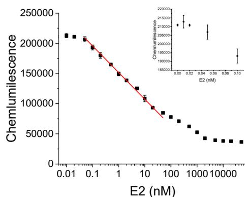
**Fig. S6** Detection of E2 by ELAA with chemiluminescence-analysis mode at optimal conditions. The inset shows the chemiluminescence signals corresponding to blank sample and low concentrations of E2. The assay buffer contained 20 mM Tris-HCl (pH 7.5), 10 mM MgCl<sub>2</sub>, 150 mM NaCl.
