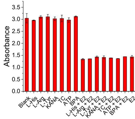
**Fig. S7** Specificity test of the assay for E2 using absorbance analysis. Blank represents the system that did not contain any analytes. The concentrations of all the analytes were 100 nM.
