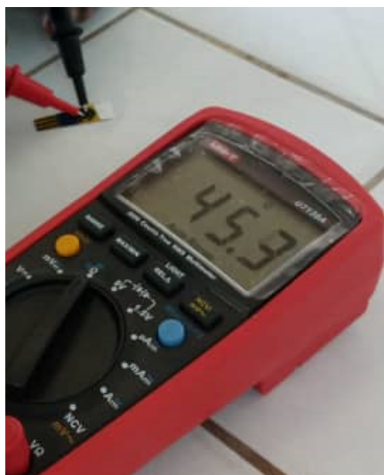
Figure S4: Measurement of the resistance of the LIGE6.4W30 electrode using a multimeter.
