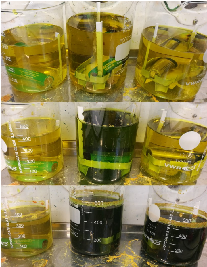
Figure S3: Three different batteries Panasonic battery, Biltema battery, and Ansmann battery respectively after discharging at (a) the same day of experiments (b) after 100 h and (c) after 250 h in redox electrolyte containing 5 wt. % electrolyte of potassium hexacyanoferrate and potassium hexacyanoferrite
