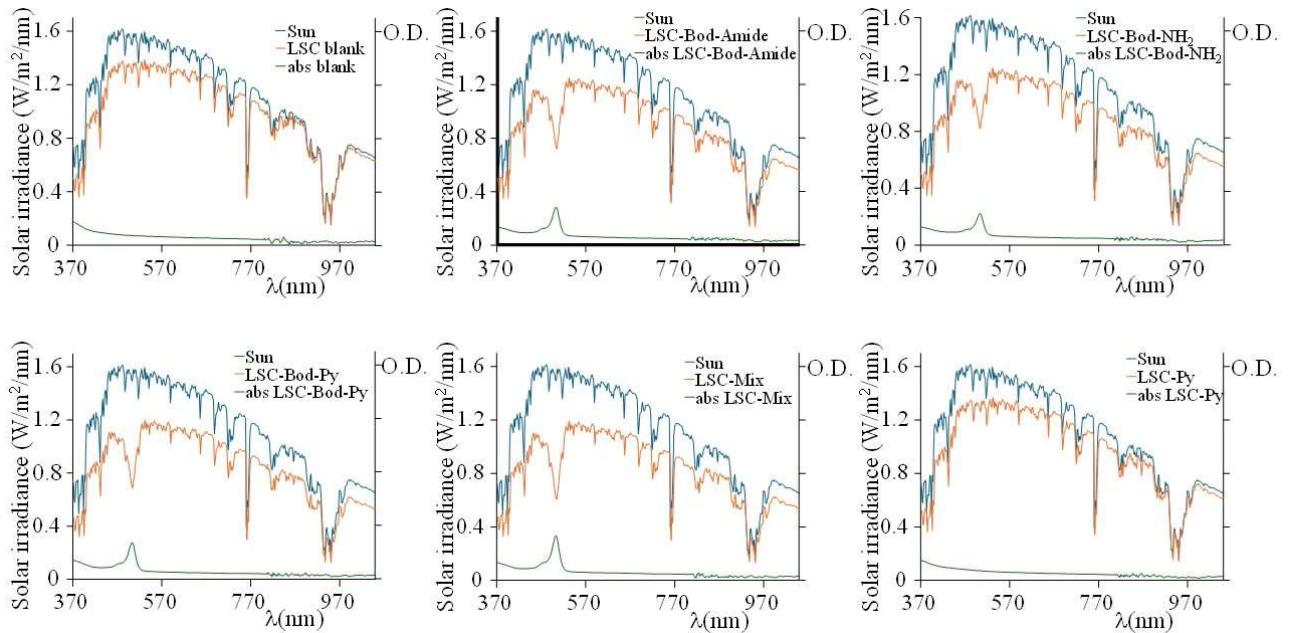
**Figure S6.** In each panel: in blue, the solar spectrum using the AM 1.5G filter; in green, the absorption spectrum; in orange, the solar spectrum filtered by the LSC.
