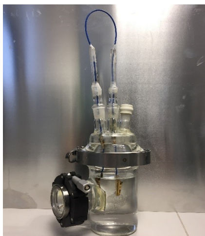
Figure S1. Custom-made reactor vessel for hydrogen evolution test with a fused silica quartz viewport. The o -YFO working electrode and Pt mesh counter electrode are connected by a single outer wire
