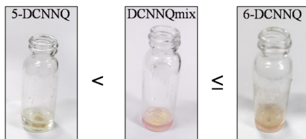
Fig. S5. Solubility tests of powder samples of 5-DCNNQ, DCNNQmix, and 6-DCNNQ in the electrolyte.
