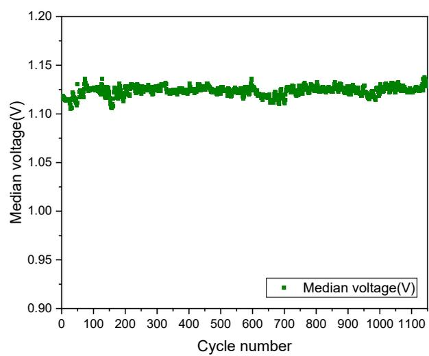
**Fig. S10** The discharge median voltage of the single cell during a 1500-hour cycling test.
