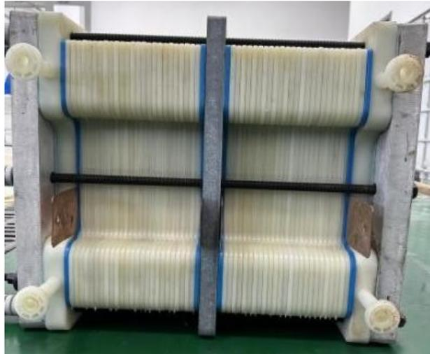
**Fig. S4 Physical view of a 52-stacked cell.**
