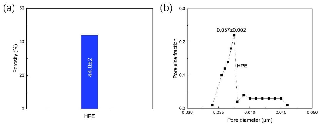
**Fig. S5 Characterizations of the HPE.** (a) Overall porosity and (b) pore size distribution of the HPE.
