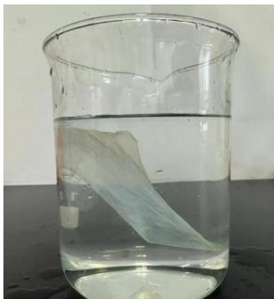
**Fig. S11 Hydrophilic stability of HPE in the single cell.** Photograph of HPE immersed in water after a 1500-hour single cell cycling test.
