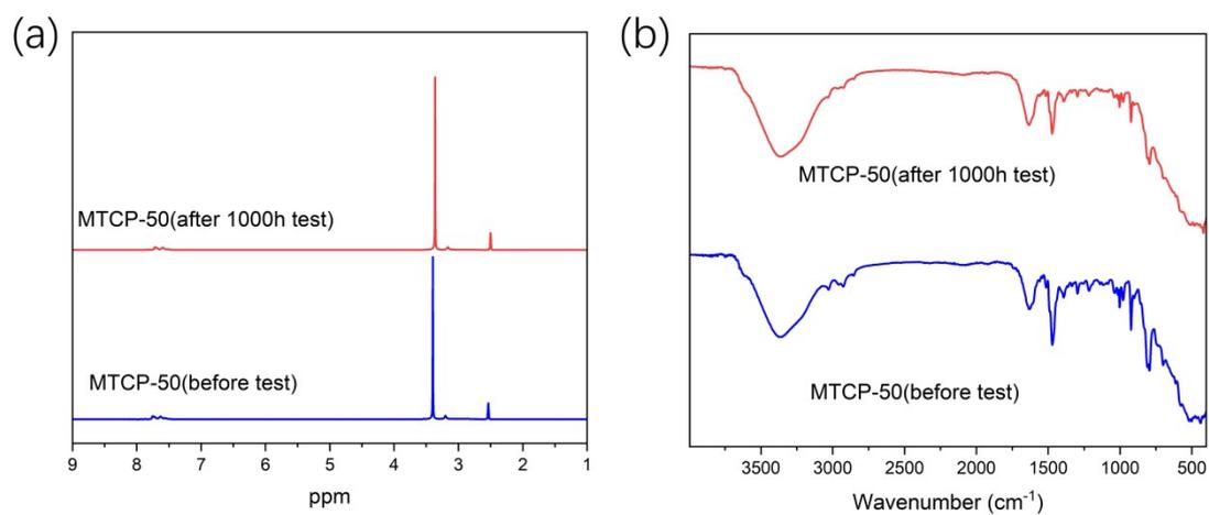
**Fig. S12 The structural integrity of AEM post post-cycling.** (a) The  $^1\text{H}$  NMR spectra and (b) FT-IR spectra of the MTCP-50 AEM before and after 1000-hour cycles.
