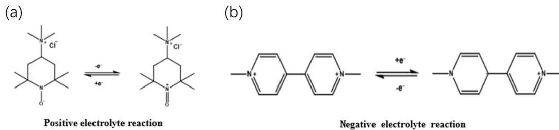
**Fig. S2 Structural details and fundamental electrode reactions of compounds.** (a) TEMPTMA (positive electrolyte) and (b) MV (negative electrolyte).
