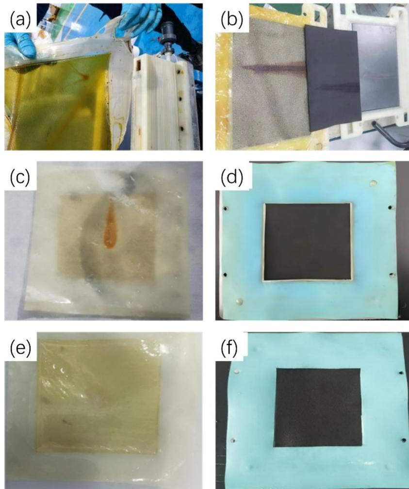
**Fig. S8 Photographs of disassembled MTCP-50 AEM.** (a) Mildly corroded MTCP-50 AEM, (b) severely corroded MTCP-50 AEM with breakage, (c) MTCP-50 AEM from a single cell with a 0.5 mm round hole after approximately 15 hours of operation, and (d) the corresponding bleached blue seal membrane (inside view). (e) Dismantled CM (MTCP-50 AEM with a 0.5 mm round hole) after approximately 90 hours of operation, and (f) the blue seal membrane without bleaching.
