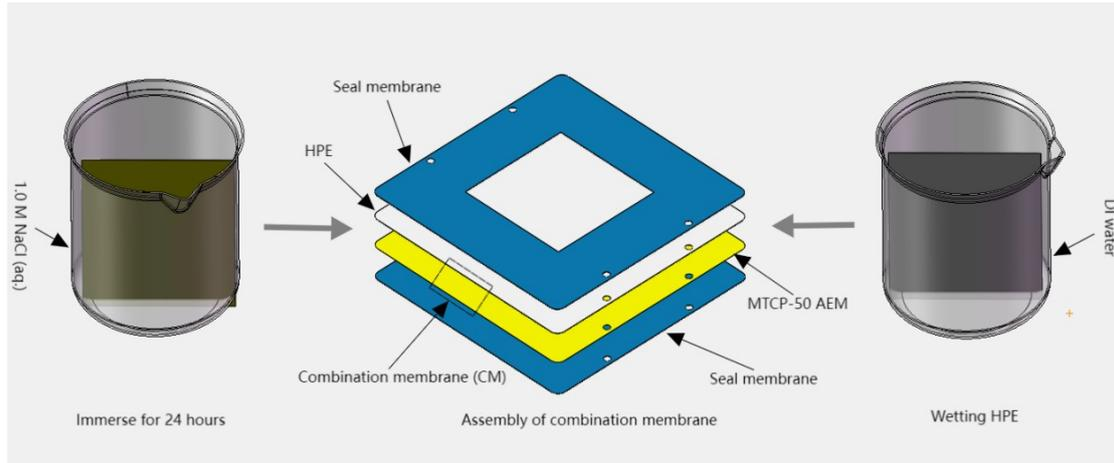
**Fig. S3 Assembly process of the CM.**
