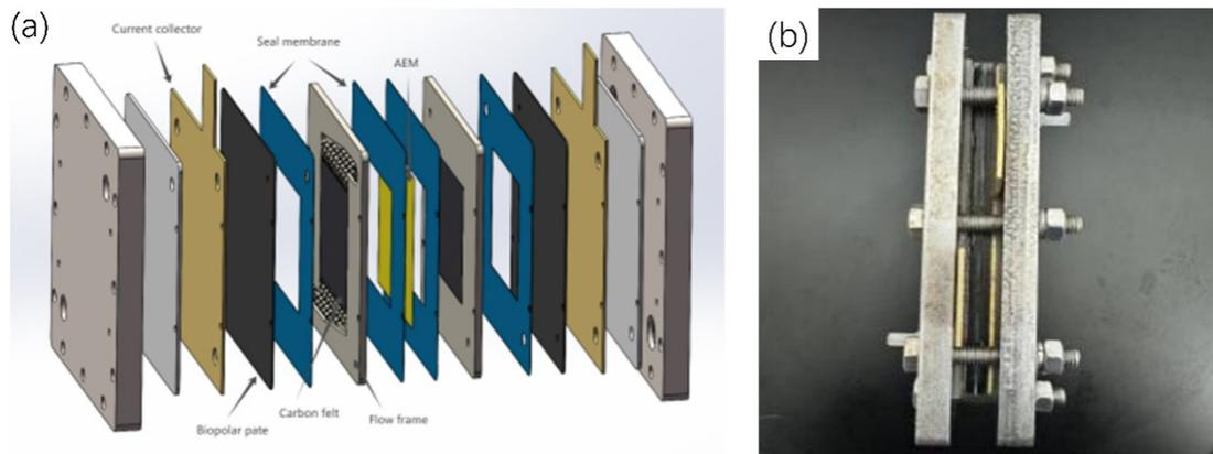
**Fig. S1 The single cell.** (a) Schematic and (b) physical views of a single cell.
