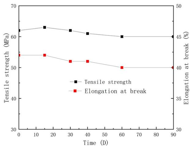
**Fig. S9** The mechanical properties of the MTCP-50 AEM with different soaking times in TEMPTMA catholyte (1.5 M, 50°C, under a 100% state of charge).
