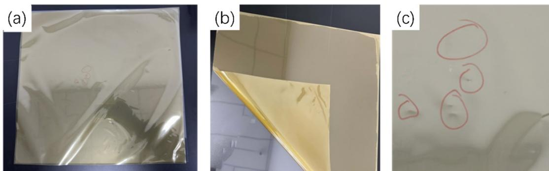
**Fig. S7 Characterizations of the MTCP-50 AEM.** The photograph of the (a) flaw areas is circled in red, which is produced during (b) the removal of the AEM from PET, and (c) the magnified view of the flaw areas.
