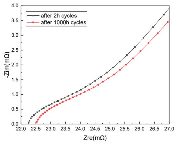
**Fig. S13 EIS measurements of the single cell with CM after 2-hour cycles and 1000-hour cycles under 50% state of charge.**
