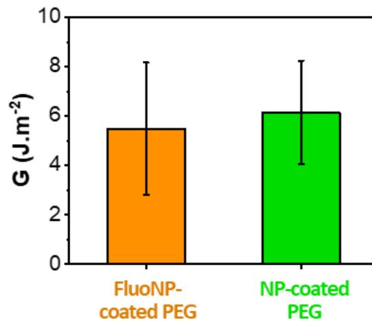
**Figure S4:** Comparison of the adhesion energy obtained with a PEG film coated with a fluorescent NP-coating (orange) and with a non-fluorescent NP-coating (green) on two samples of the same freshly dissected liver (i.e. same level of tissue hydration  $H$  in both cases).
