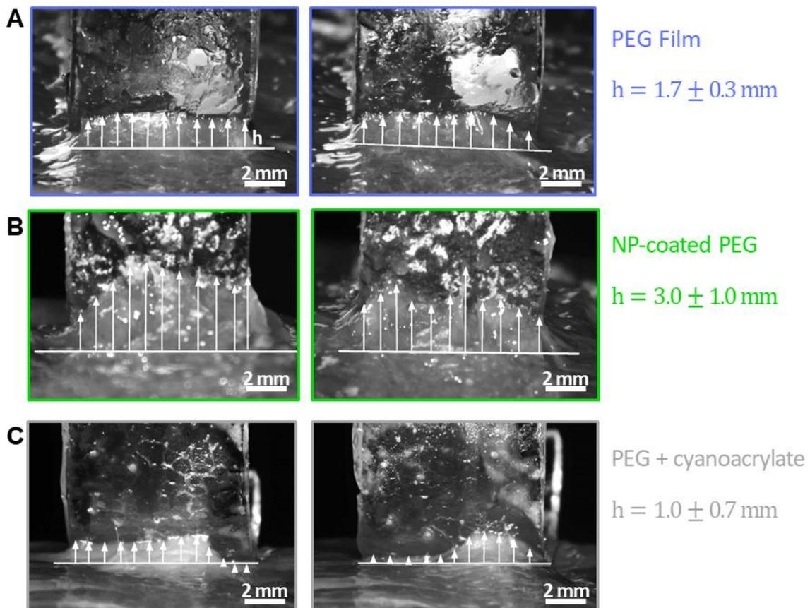
**Figure S2:** Measurement of the height  $h$  of the detachment line above the plane of the film-tissue interface during steady-state peeling in the case of a bare PEG film (A), an NP-coated PEG film (B) and a PEG film covered with medical grade cyanoacrylate (C). Measurements of  $h$  were performed on at least 50 different locations (represented by the white arrows) randomly selected over at least 4 different snapshots of the peeling front of each system.
