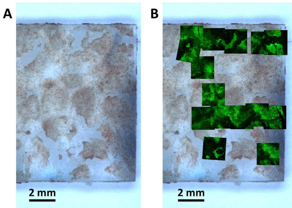
**Figure S5:** (A) Photograph a PEG film coated with a fluorescent NP-coating after peeling in the adhesive regime ( $v_{abs}/v_{free} > 1$ ) on a freshly dissected liver sample. (B) Same photograph displaying superimposed fluorescent micrographs taken in some areas. These observations show that the areas where liver tissue was transferred correspond to areas where the fluorescent NP-coating is still present on the PEG surface after peeling.
