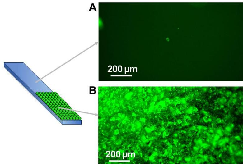
**Figure S6:** Fluorescent micrographs of an uncoated (A) and NP-coated (B) PEG film before peeling.
