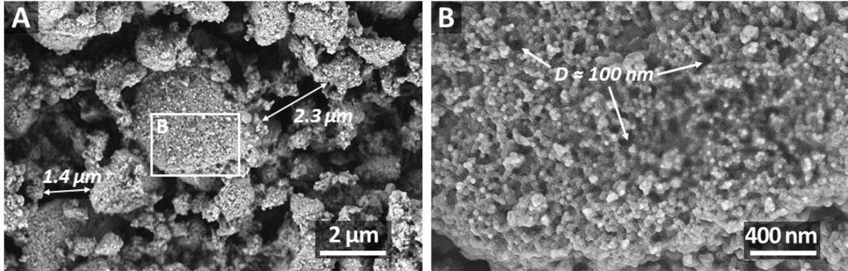
**Figure S3:** SEM images of the NP coating on which the size of pores is displayed. In particular, the image (A) show microscopic inter-aggregate porosities while image (B) displays intra-aggregate porosities in the submicron range. From these images the coating porosities is roughly estimated to be of the order of 0.1 to 10  $\mu\text{m}$ .
