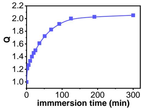
**Figure S1:** Swelling ratio of a 1 mm-thick PEG film as a function of immersion time in water.
