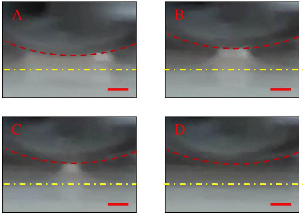
Figure S3: Evolution of the vertical extension viewed from the side for  $V_u = 10$  mm/s and  $t_{\text{dwell}} = 0.5$  s case at the instant of (A) pull-off, (B) and (C) right before the full separation, and (D) right after the full separation. The red dashed lines denote the contour of the probe, while the yellow dashed lines represent the baseline of the vertical extension. (Scale bar: 1 mm)
