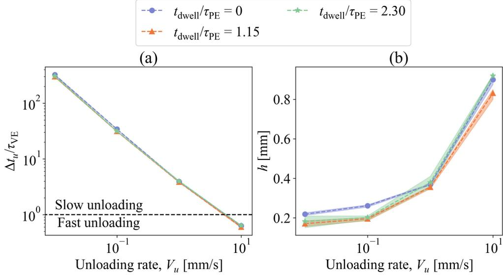
Figure S2: (a) The duration of unloading, from the start of unloading to full separation, normalized by the viscoelastic relaxation time  $\Delta t_u / \tau_{VE}$ . (b) The estimated vertical extension  $h$ . The shaded area in both figures represents the range between the maximum and minimum values.
