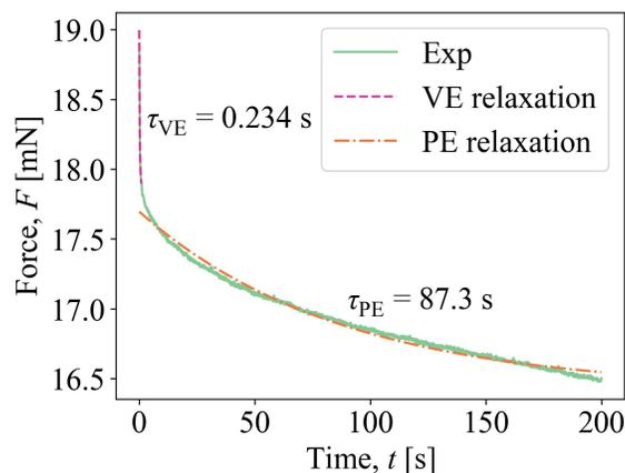
Figure S1: Representative relaxation curve from the adhesion experiments with a holding time of  $t_{\text{dwell}} = 200 \text{ s}$ . The curve illustrates two relaxation time constants:  $\tau_{\text{VE}}$ , which covers the initial relaxation from 0 to 1 s, and  $\tau_{\text{PE}}$ , which captures the broader range of relaxation from 0 to 200 s.
