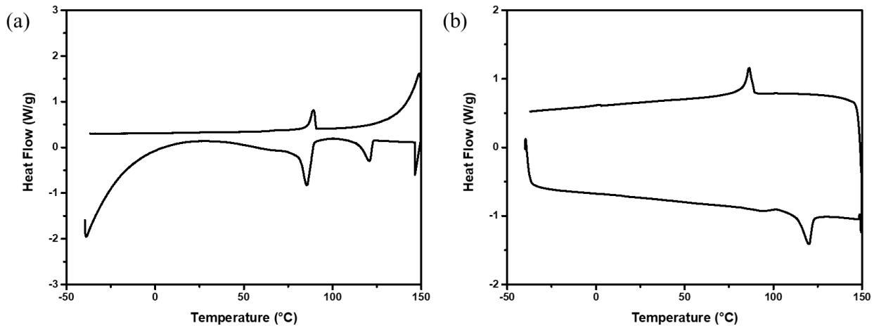
Figure S23. DSC thermograms of DBP(CA,12) for the (a) first and (b) second heating/cooling cycles.
