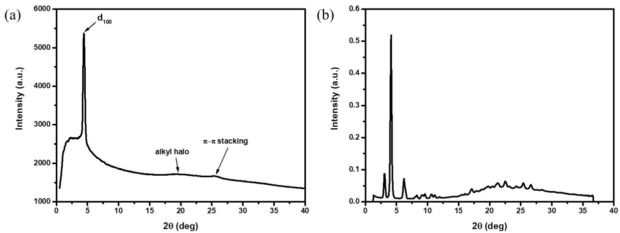
**Figure S46.** X-ray diffractograms of **DBP(PrOH,12)** at (a) 106 °C on the Rigaku instrument and (b) room temperature on the SAXS instrument.
