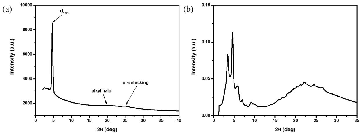
**Figure S45.** X-ray diffractograms of **DBP(PrOH,6)** at (a) 188 °C on the Rigaku instrument and (b) room temperature on the SAXS instrument.
