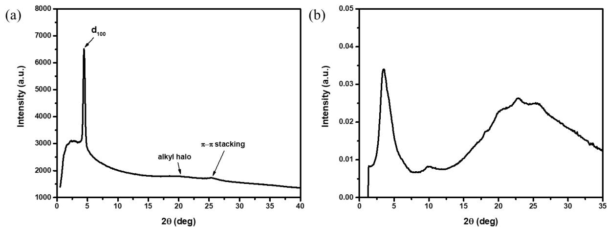
**Figure S41.** X-ray diffractograms of **DBP(Me,12)** at (a) 104 °C on the Rigaku instrument and (b) room temperature on the SAXS instrument.
