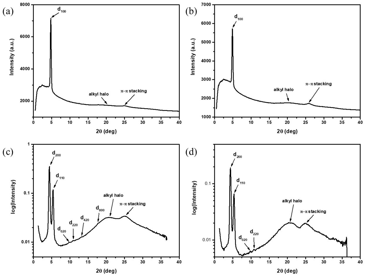
**Figure S48.** X-ray diffractograms of **dDBP(6)** at (a) 171 °C and (b) room temperature on the Rigaku instrument, and (c) 2 years and (d) 5 years at room temperature on the SAXS instrument.
