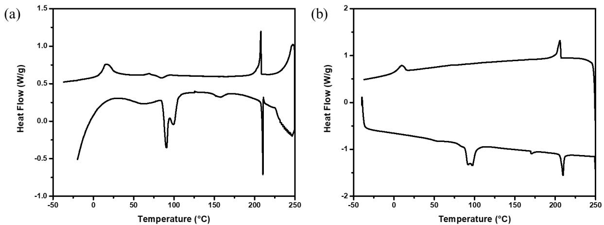
Figure S24. DSC thermograms of DBP(PrOH,1) for the (a) first and (b) second heating/cooling cycles.
