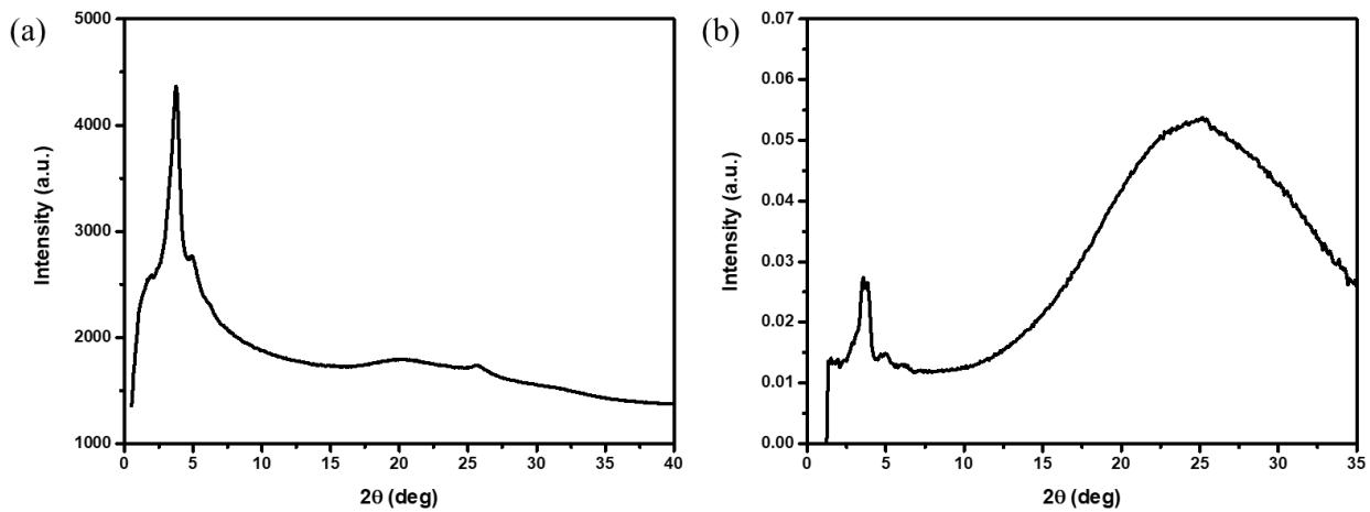
**Figure S43.** X-ray diffractograms of **DBP(CA,12)** at room temperature on (a) the Rigaku instrument and (b) the SAXS instrument.
