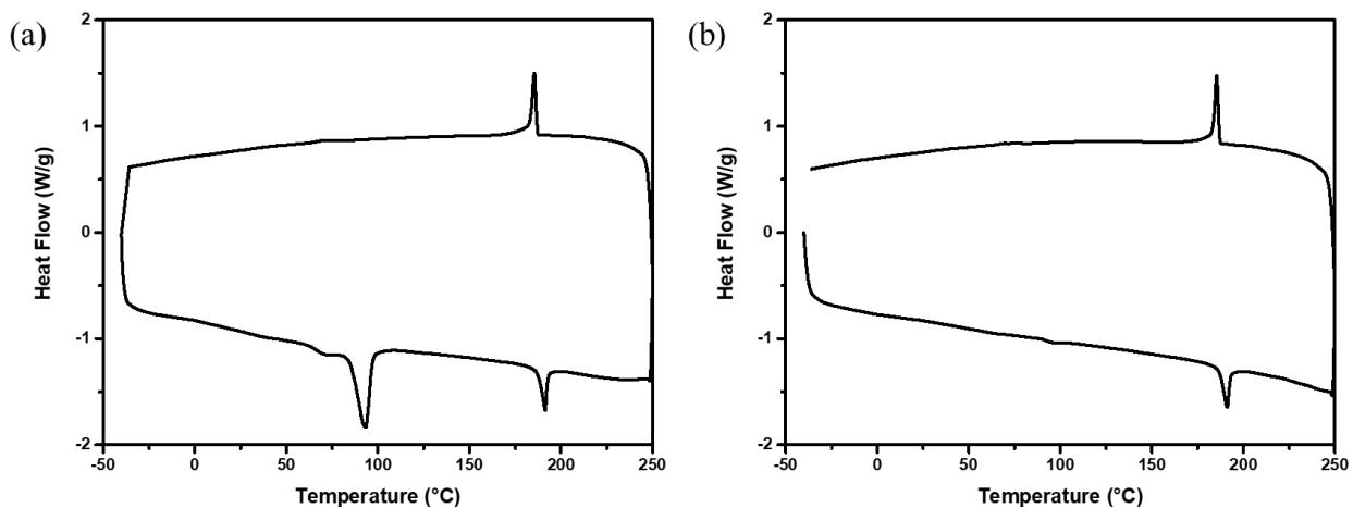
**Figure S28.** DSC thermograms of dDBP(6) for the (a) first and (b) second heating/cooling cycles.
