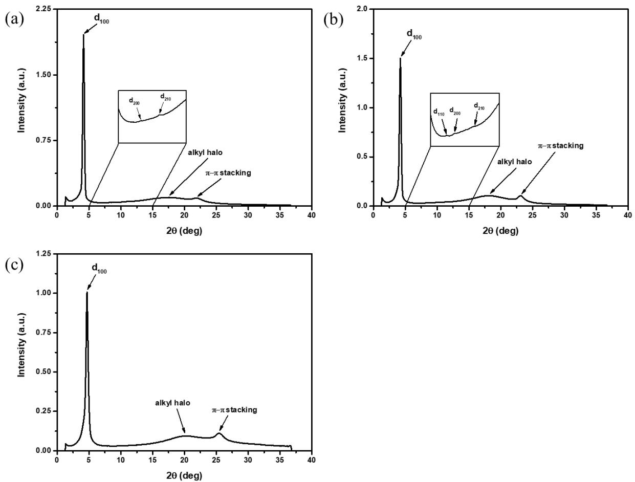
**Figure S50.** X-ray diffractograms of **dDBP(hyd,6)** at (a)  $270^{\circ}\text{C}$ , (b) room temperature, and (c) 10 months at room temperature. All measurements were performed on the SAXS instrument.
