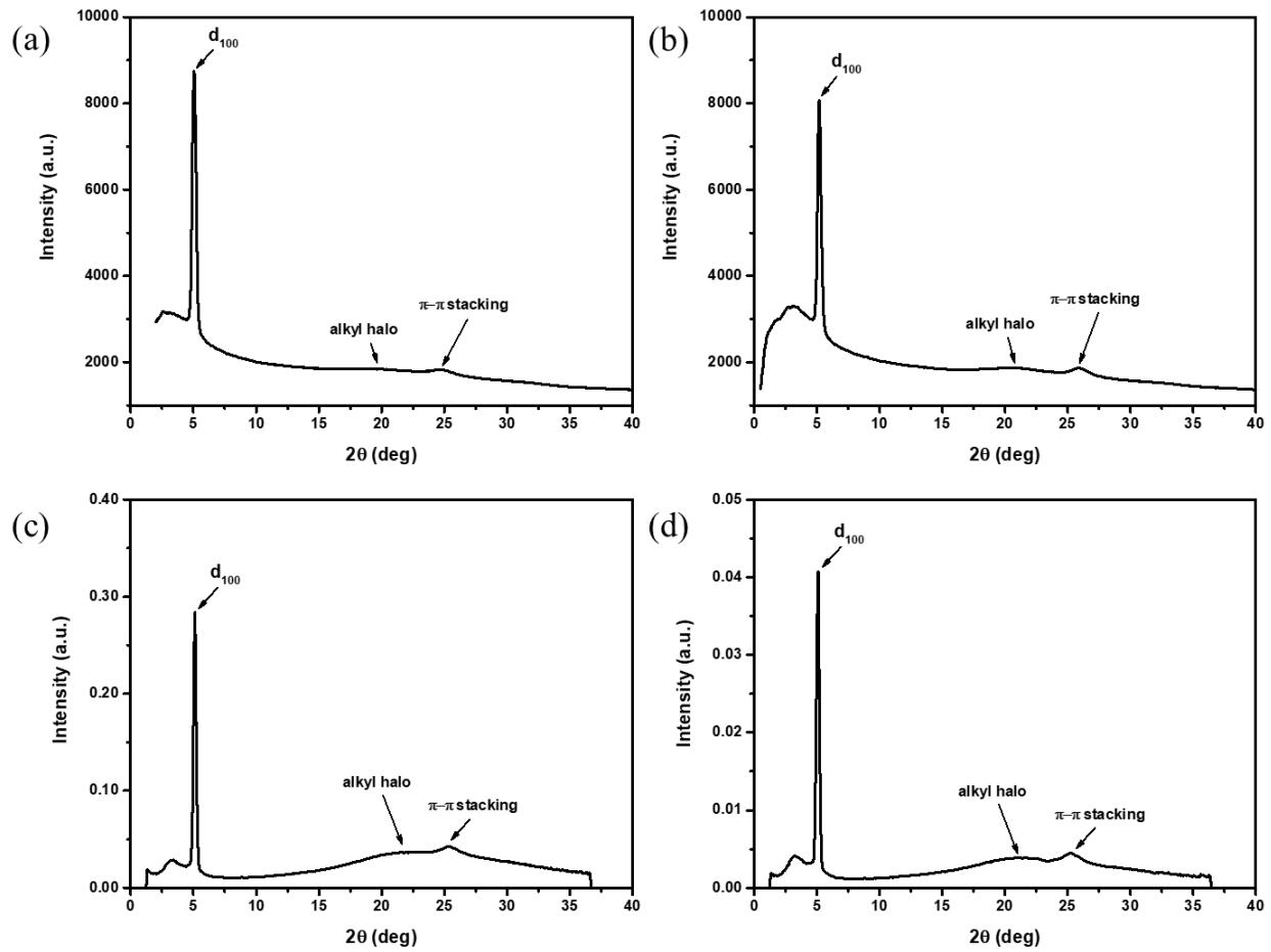
**Figure S47.** X-ray diffractograms of **dDBP(1)** at (a) 193 °C and (b) room temperature on the Rigaku instrument, and (c) 2 years and (d) 5 years at room temperature on the SAXS instrument.
