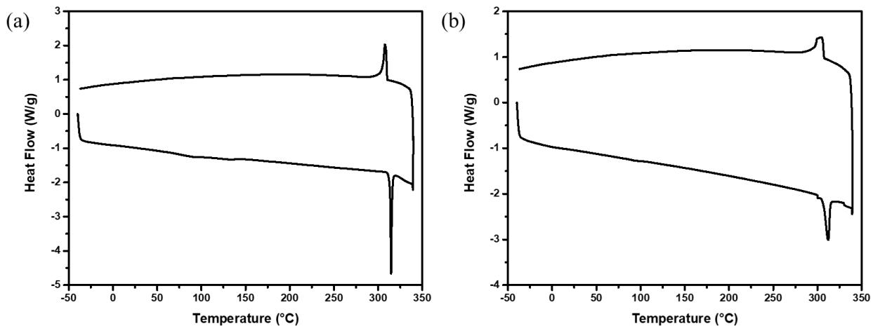
**Figure S30.** DSC thermograms of **dDBP(hyd,6)** for the (a) first and (b) second heating/cooling cycles.
