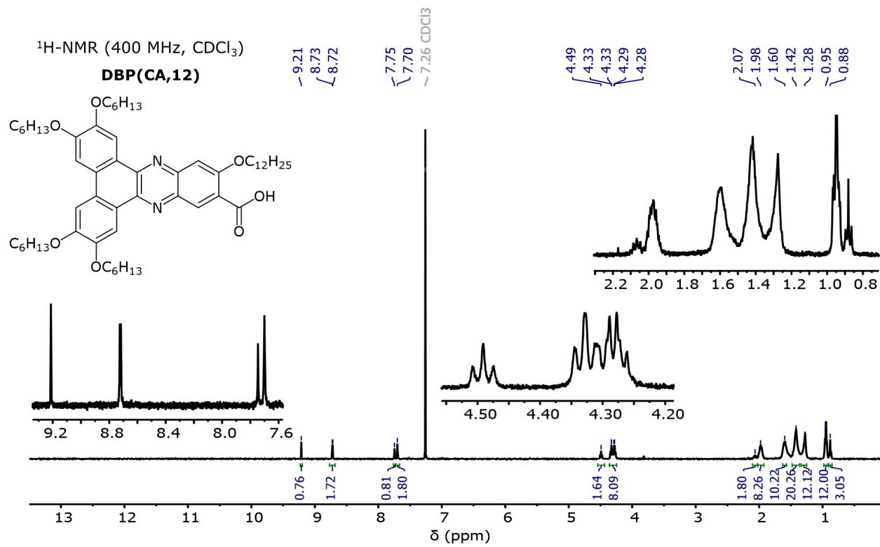
Figure S5. <sup>1</sup>H-NMR spectrum of DBP(CA,12).
