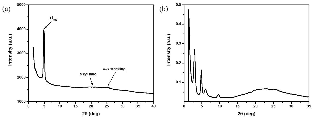
**Figure S44.** X-ray diffractograms of **DBP(PrOH,1)** at (a) 178 °C on the Rigaku instrument and (b) room temperature on the SAXS instrument.
