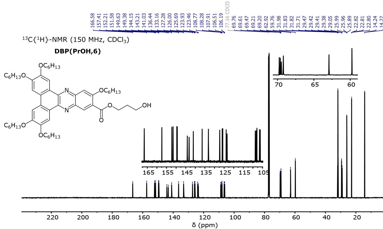
Figure S10. <sup>13</sup>C{<sup>1</sup>H}-NMR spectrum of DBP(PrOH,6).
