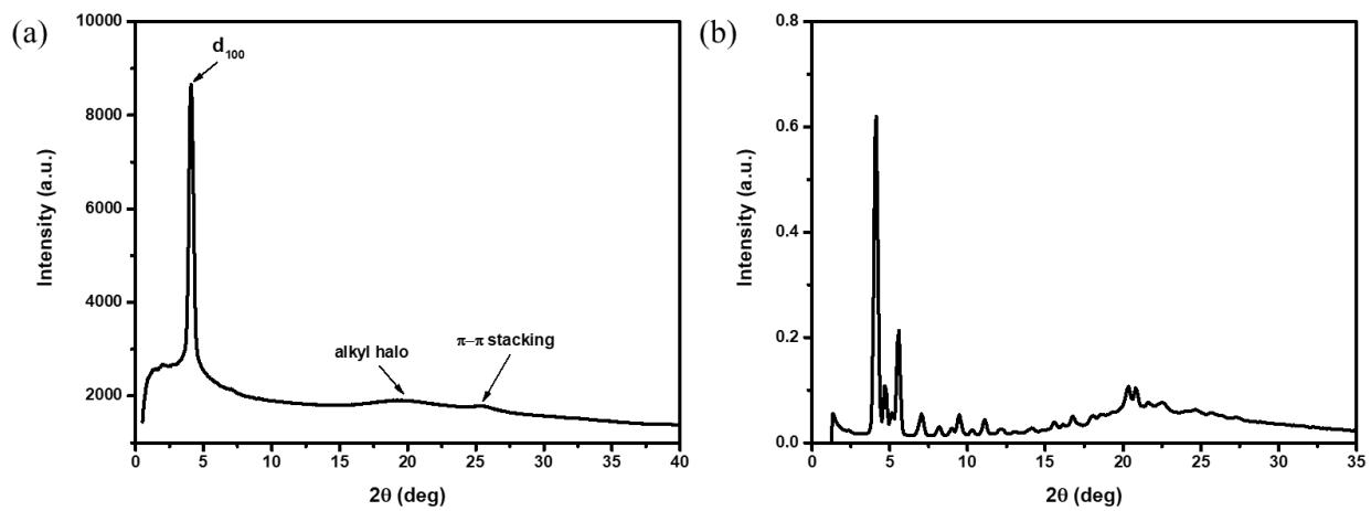
**Figure S42.** X-ray diffractograms of **DBP(Dod,12)** at (a) 95 °C on the Rigaku instrument and (b) room temperature on the SAXS instrument.
