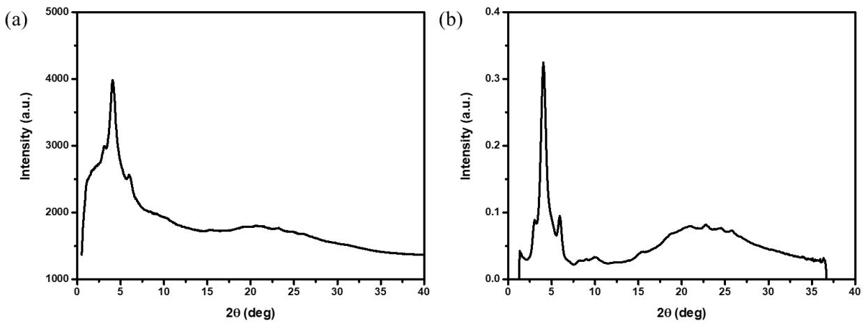
**Figure S49.** X-ray diffractograms of **dDBP(12)** at room temperature on (a) the Rigaku instrument and (b) the SAXS instrument.
