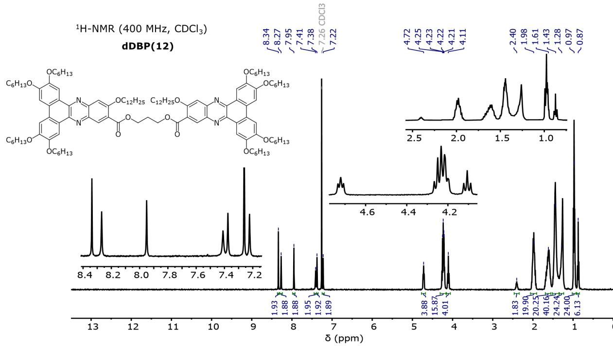
**Figure S17.** <sup>1</sup>H-NMR spectrum of dDBP(12).
