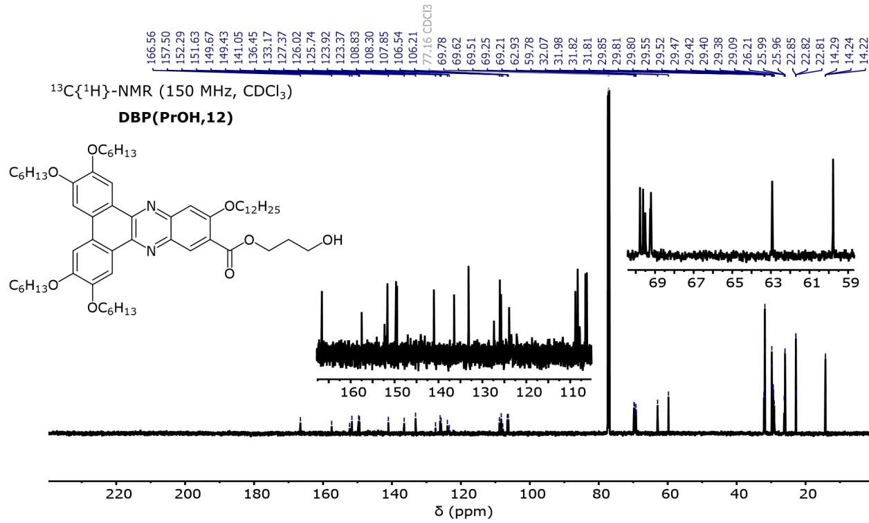
Figure S12. <sup>13</sup>C{<sup>1</sup>H} NMR spectrum of DBP(PrOH,12).
