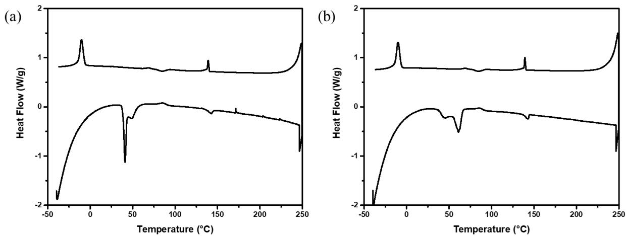
Figure S21. DSC thermograms of DBP(Me,12) for the (a) first and (b) second heating/cooling cycles.
