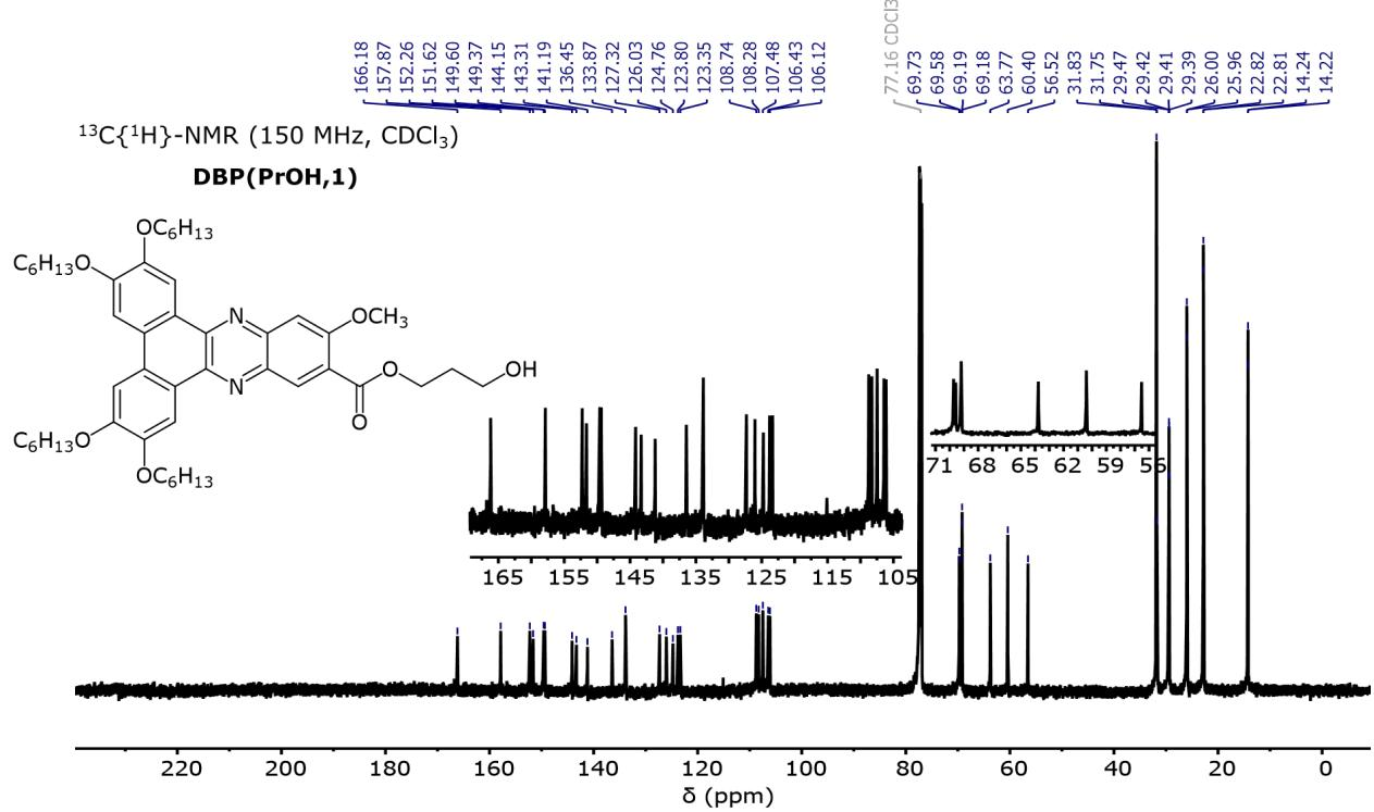
Figure S8. <sup>13</sup>C{<sup>1</sup>H}-NMR spectrum of DBP(PrOH,1).
