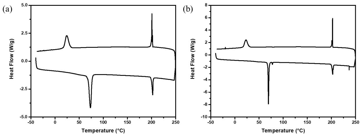
Figure S25. DSC thermograms of DBP(PrOH,6) for the (a) first and (b) second heating/cooling cycles.
