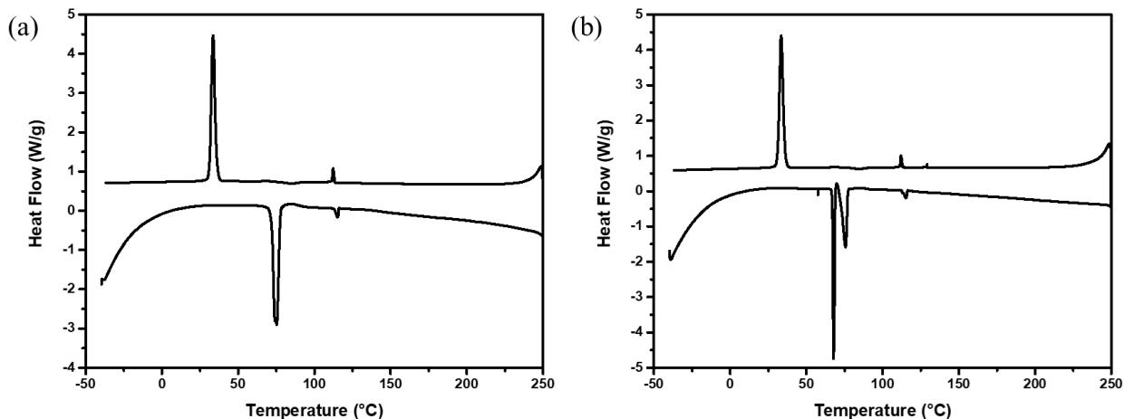
Figure S22. DSC thermograms of DBP(Dod,12) for the (a) first and (b) second heating/cooling cycles.
