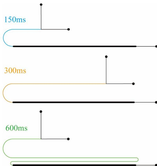
**Fig. S2.** Schematic diagrams of microfluidic chips that have three aging times. (The lengths of the narrow channels in blue, orange, and green are 23.3mm, 46.7mm, and 93.3mm, respectively)
