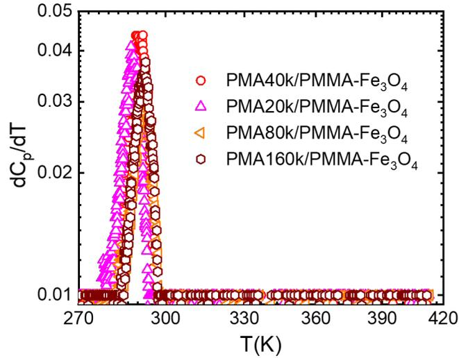
**Figure S2.** Temperature derivative of the specific heat capacity,  $dC_p/dT$ , of the PMA/PMMA-g- $Fe_3O_4$  nanocomposites. Only one  $T_g$  is observed for all nanocomposites.
