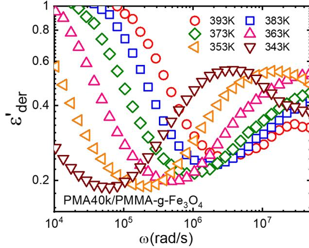
**Figure S4.** Derivative spectra,  $\epsilon'_{der}$ , of PMA40k/PMMA-g-Fe<sub>3</sub>O<sub>4</sub> at different temperatures 393K (red circles), 383K (blue squares), 373K (olive diamonds), 363K (pink triangles), 353K (orange left triangles), 343K (wine inverted triangles).
