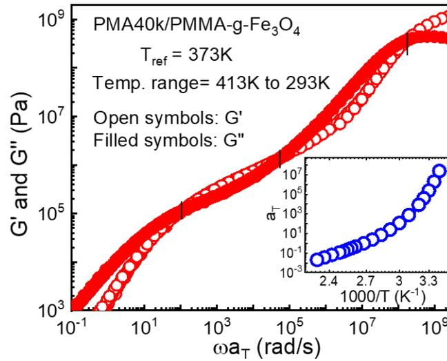
**Figure S5.** Linear viscoelastic master curve of PMA40k/PMMA-g-Fe<sub>3</sub>O<sub>4</sub>,  $G'$  (open red circles) and  $G''$  (filled red circles), at a reference temperature of 373K. The inset provides the dynamics shift factor,  $a_T$ , from the rheological measurements. No vertical shift is needed for the construction of the master curve. No signs of  $\alpha$  relaxation of PMMA can be detected from the rheological measurements
