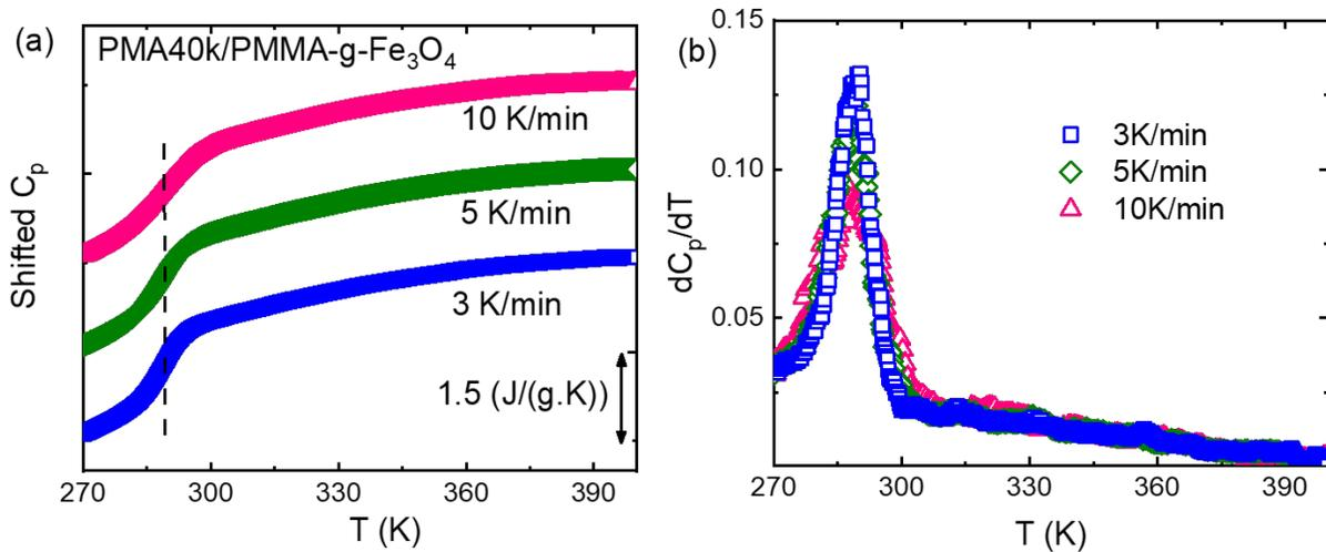
**Figure S3.** (a) Shifted heat capacity,  $C_p$ , and (b) the temperature derivative of the specific heat capacity,  $dC_p/dT$ , of PMA40k/PMMA-g- $Fe_3O_4$  composite at cooling rates of 3K/min (blue squares), 5K/min (olive diamonds), 10K/min (pink upper triangles).
