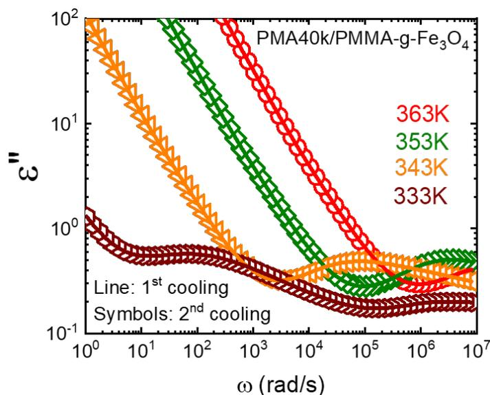
**Figure S1.** Dielectric loss permittivity  $\varepsilon''(\omega)$  for PMA40k/PMMA-g-Fe<sub>3</sub>O<sub>4</sub> at 363K (red circles), 353K (olive diamonds), 343K (orange left triangles), 333K (wine hexagons): the lines represent the spectra at first cooling and the symbols represent the spectra at second cooling (symbols). For each comparison, at least two tests have been performed on different specimen.
