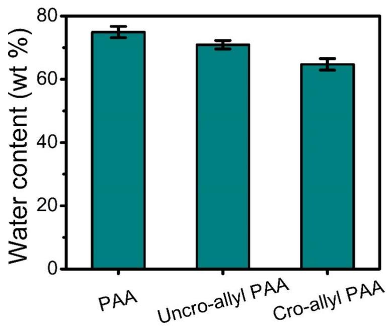
**Figure S9.** Water content (wt%) of BPEI-PAA coacervate, uncrosslinked BPEI-allyl-PAA coacervate and crosslinked BPEI-allyl-PAA coacervate. The coacervate samples were prepared with an initial pH of 6.5 and a 1:1 molar ratio of BPEI to PAA or allyl-PAA. The error bars represent the standard deviation of 3-5 measurements
