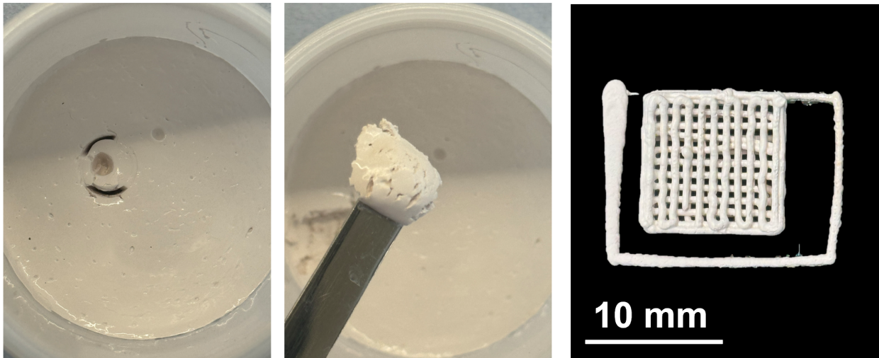
Figure 10: Adding G \delta L to a stable STO emulsion gel (to trigger a controlled assembly through inter macro-molecular hydrogen bond formation) leads to a very heterogeneous formulations with signs of microstructure disruption (e.g. phase separation, aggregates and macroscopic cracks).
