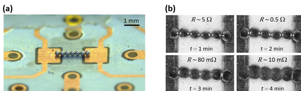
**Figure S1.** (a) Image showing a particle chain of 300- $\mu\text{m}$  Sn<sub>63</sub>Pb<sub>37</sub> spheres on a PCB carrier, stretched between two copper pads. (b) Top-view images of the compressed chain at four different stages, corresponding to 3%, 6%, 22%, and 50% compressive strain, during which the resistance of the structure changes from 5  $\Omega$  to 10 m $\Omega$ .
