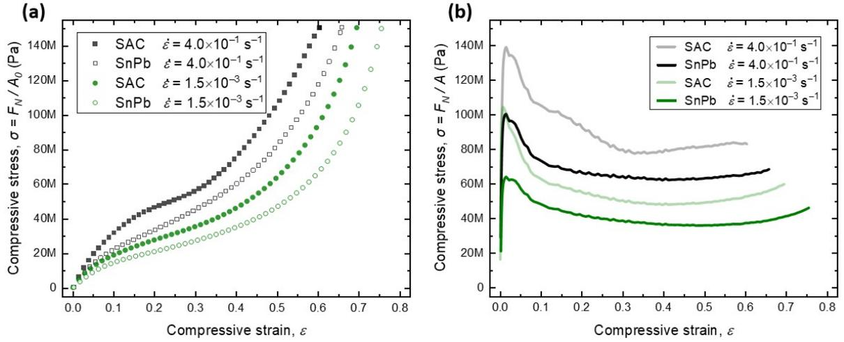
**Figure S3.** Compressive stress-strain curves for leaded and unleaded solder balls (a) Stress is calculated as applied force divided by the initial (equatorial) cross-sectional area of the uncompressed sphere. (b) Stress is presented as force divided by the actual contact area between the compressive slab and the sphere, which corresponds to a classical pressure-based approach.
