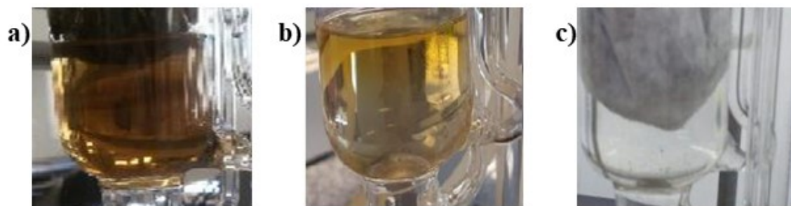
Figure S1: Appearance of the acetone used in the first washing of the SC prepared a) OL (3) 0.25h-180, b) OSE (1) 0.25h-120 and c) OSE (3) 6h-180.
