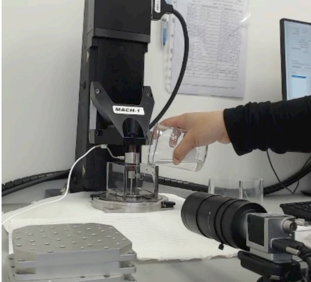
Fig. S4 | Image of mechanical characterization setup. Yeast-laden hydrogel capsules are lightly held between the load cell and the base of the instrument and water is poured into the gap to keep the capsules hydrated. Experiments are then performed as described in methods.
