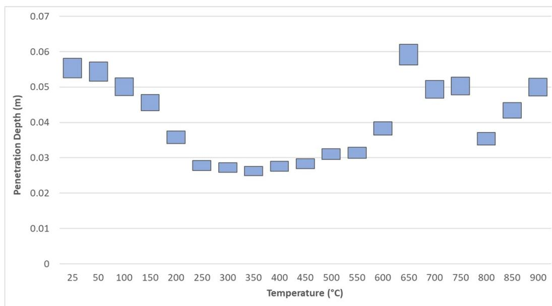
Fig. S1: Interval of MW penetration depth calculated for a spent LCO battery BM, containing 20% of graphite. Each blue rectangle represents an interval, showing the variability in the MW penetration depth for each temperature, depending on the BM density and dielectric parameters.
