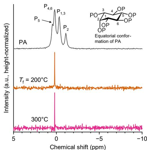
**Figure S4.** <sup>31</sup>P solution NMR spectrum of PA (aqueous standard solution) and aqueous extracts from char after pyrolysis of cellulose loaded with 1.0 wt% PA at 200°C and 300°C. P = -PO<sub>3</sub>H<sub>2</sub>, -PO<sub>3</sub>H<sup>-</sup>, or -PO<sub>3</sub><sup>2-</sup>, depending on pH.<sup>50</sup>
