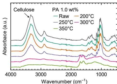
**Figure S2.** Fourier transform infrared spectroscopy (FT-IR) of cellulose loaded with 1.0 wt% PA after pyrolysis at different temperatures. FT-IR analysis was carried out in an attenuated total reflectance (ATR) mode on a PerkinElmer Spectrum two.
