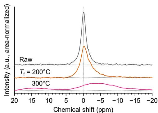
**Figure S5.**  $^{31}\text{P}$  solid-state NMR spectrum of chars prepared by pyrolysis of cellulose loaded with 1.0 wt% phosphoric acid at different temperatures.
