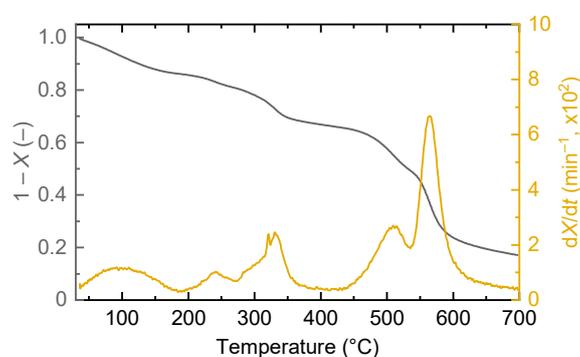
**Figure S3.** TGA of PA under a flow of N<sub>2</sub> at 10 °C/min. PA contained about 20 wt% of water, which was lost below 200°C.
