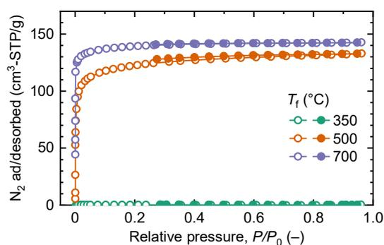
**Figure S7.**  $\text{N}_2$  ad/desorption isotherms of chars prepared at different  $T_f$ . BET surface area calculated from the isotherms were 1.0, 472, and 550  $\text{m}^2/\text{g}$  for chars prepared at 350, 500, and 700°C, respectively.
