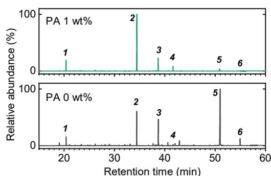
**Figure S8.** GC/MS chromatogram of liquid product from slow pyrolysis of cellulose loaded with 1.0 wt% PA and without PA: 1) furfural, 2) LGO, 3) DGP, 4) ADGH, 5) LGA, and 6) AGF.
