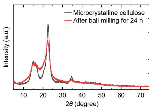
**Figure S6.** XRD patterns of cellulose before and after ball-milling. CrI decreased from 85.6% to 60.0% with the ball-milling.
