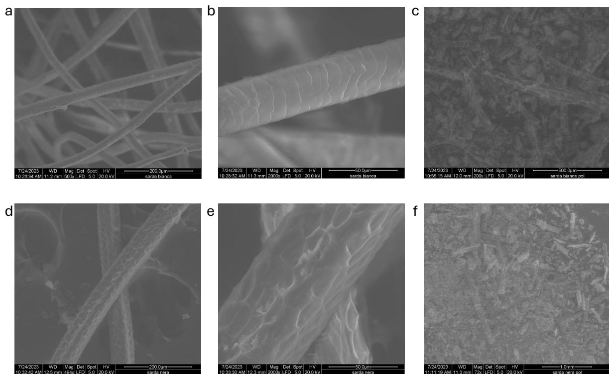
**Figure 1.** SEM images for wool samples before and after the treatment; a) White Wool Fibre (WWF); b) White Wool Fibre (WWF) – magnification; c) White Wool Powder (WWP); d) Black Wool Fibre (BWF); e) Black Wool Fibre (BWF) – magnification; f) Black Wool Powder (BWP).
