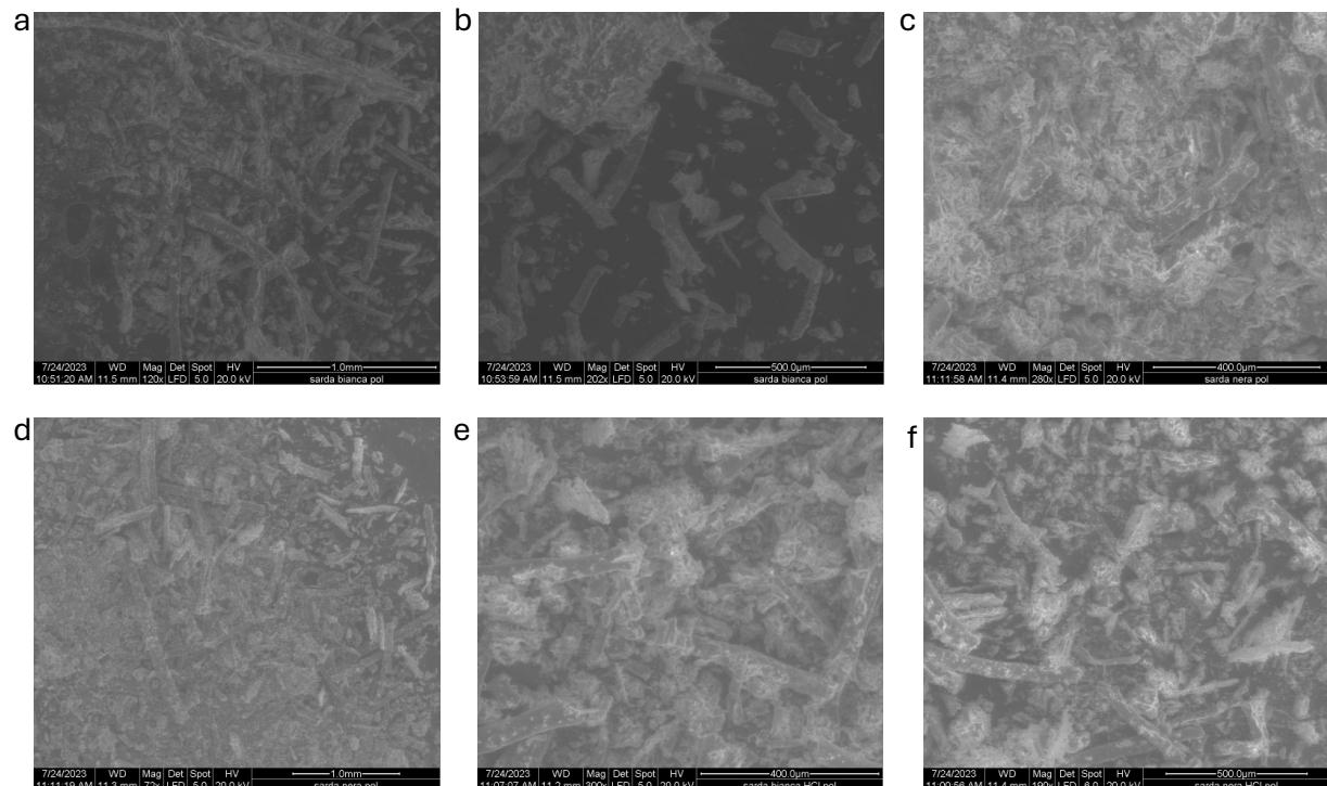
**Figure 2.** SEM images for wool powder samples with and without HCl treatment; a) White Wool Powder (WWP); b) White Wool Powder (WWP) – magnification; c) White Wool Powder-HCl (WWP-HCl); d) Black Wool Fibre (BWP); e) Black Wool Powder (BWP) – magnification; f) Black Wool Powder- HCl (BWP-HCl).
