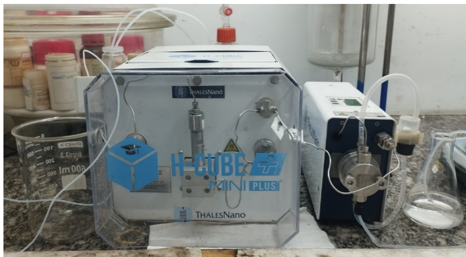
Figure S3: H-Cube ® Mini Plus continuous flow hydrogenation reactor (ThalesNano).
