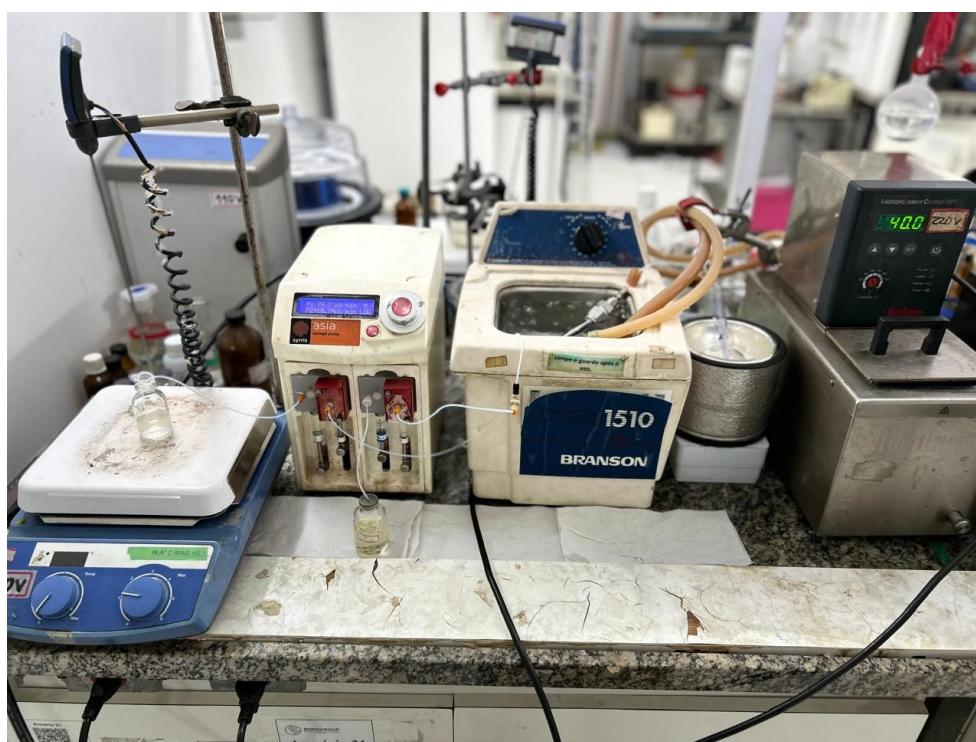
Figure S1: Setup for continuous flow hydrolysis.
