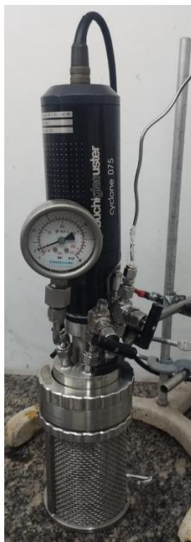
Figure S2: Pressure reactor - miniclave drive - Buchiglas (Büchi AG –Switzerland).
