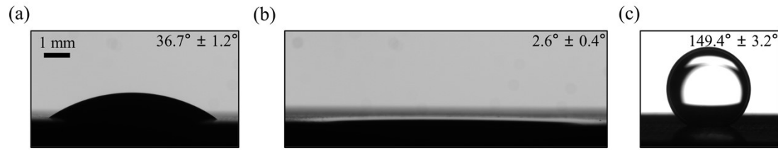
Fig. S1 Contact angle of (a) water in air, (b) silicone oil in air, and (c) water under silicone oil. The silicone oil is of 10 mPa·s, and the substrate is the 3D-printed resin sample used in the experiments in Fig. 1, 2 and 3. The data are shown as mean \pm SD ( N = 3 ).
