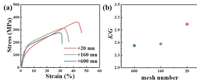
Fig. S2 (a) Stress-strain curves and (b) calculated  $K/G$  of  $\text{Mg}_{3.1}\text{Bi}_{1.5}\text{Sb}_{0.49}\text{Te}_{0.01}$  samples with different particle size.
