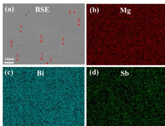
Fig. S3 (a) SEM image and corresponding EDS composition mapping of (b) Mg, (c) Bi, (d) Sb elements of  $\text{Mg}_{3.1}\text{Bi}_{1.5}\text{Sb}_{0.49}\text{Te}_{0.01}$ .
