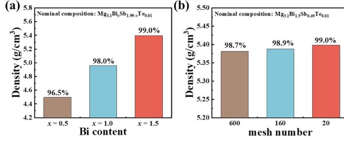
**Fig. S7** Measured densities of the samples of (a) Mg<sub>3.1</sub>Bi<sub>x</sub>Sb<sub>1.99-x</sub>Te<sub>0.01</sub> ( $x = 0.5, 1.0, 1.5$ ) and (b) Mg<sub>3.1</sub>Bi<sub>1.5</sub>Sb<sub>0.49</sub>Te<sub>0.01</sub> with different particle size. The relative densities of all the samples are marked above the columns.
