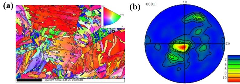
**Fig. S4** (a) Orientation imaging microscopy map and (b) pole figure of (0001) plane obtained from EBSD analysis of +20 nm sample.
