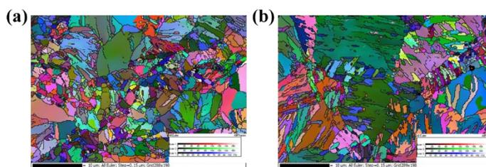
Fig. S1 EBSD images of  $\text{Mg}_{3.1}\text{Bi}_{1.5}\text{Sb}_{0.49}\text{Te}_{0.01}$  (a) +600 mn sample and (b) +20 mn sample.
