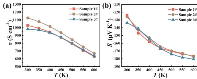
**Fig. S6** Measurement results of (a) electrical conductivity, (b) Seebeck coefficient of the reproduced +20 nm samples.
