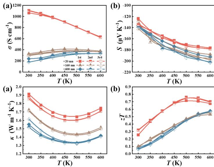
**Fig. S5** Repeated tests of (a) electrical conductivity (b) Seebeck coefficient (c) thermal conductivity and (d) calculated  $zT$  of  $\text{Mg}_{3.1}\text{Bi}_{1.5}\text{Sb}_{0.49}\text{Te}_{0.01}$  samples in 1F.
