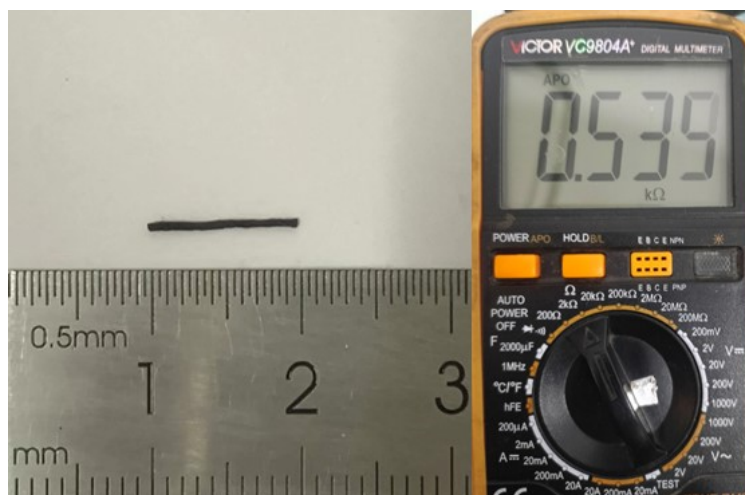
Fig. S7 Resistance value of 150@GR/TPU fibrous yarn with a length of 1cm.
