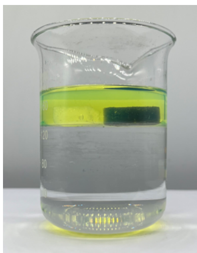
Fig. S10 Photographs of PLA (left) and G-PLA (right) aerogel in diesel/water mixture.
