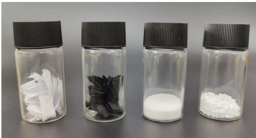
**Figure S14.** Images of PET fibers, dyed PET fibers, PET powder (0.15 mm particle size) and PET particles (5 mm particle size).
