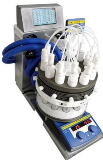
Figure S1. Schematic view of WP-TEC-1020HSL of WATTCAS photoreactor instrument for the photocatalytic measurements.
