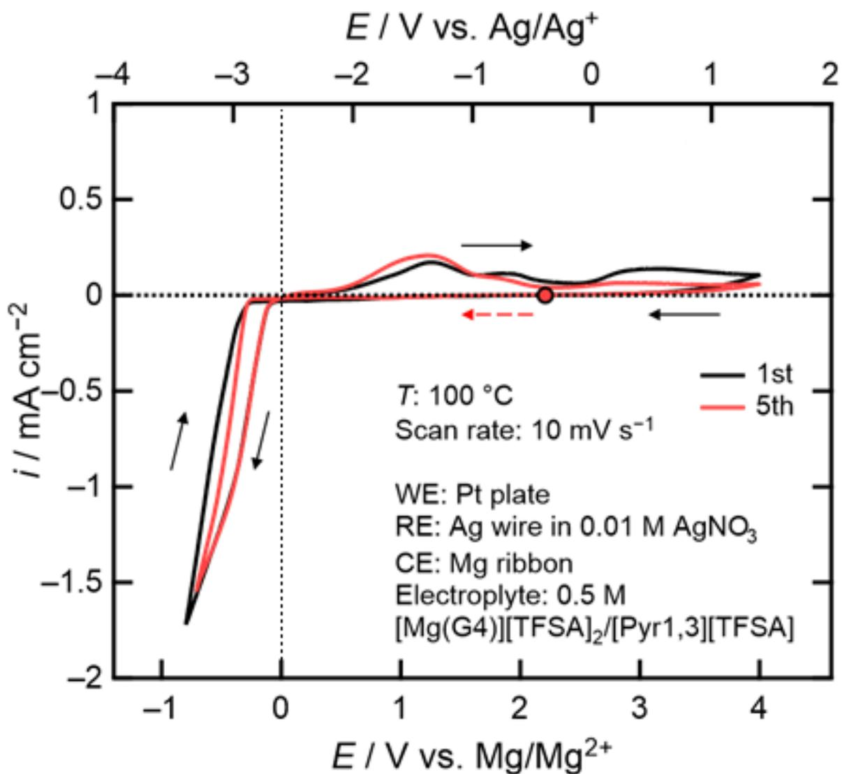
**Figure S2.** Cyclic voltammogram with Pt working electrode measured at a scan rate  $10 \text{ mV s}^{-1}$  at  $100 \text{ }^\circ\text{C}$ . The potential at which Mg deposition and dissolution were observed, denoted with the dotted line above, was used to determine the conversion from the  $\text{Ag}/\text{Ag}^+$  reference to  $\text{Mg}/\text{Mg}^{2+}$ :  $0 \text{ V vs. Mg}/\text{Mg}^{2+} = -2.6 \text{ V vs. Mg}/\text{Mg}^{2+}$ .
