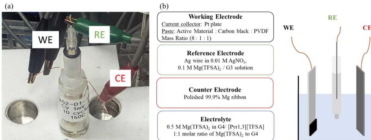
**Figure S1.** (a) Picture of the three-electrode beaker cell used for electrochemical measurements, (b) schematic diagram of the three-electrode beaker cell setup with details regarding individual components.
