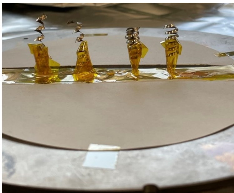
Figure S14: A photograph of a tailor-made sample holder for Pt atoms deposition on the swarf surface.
