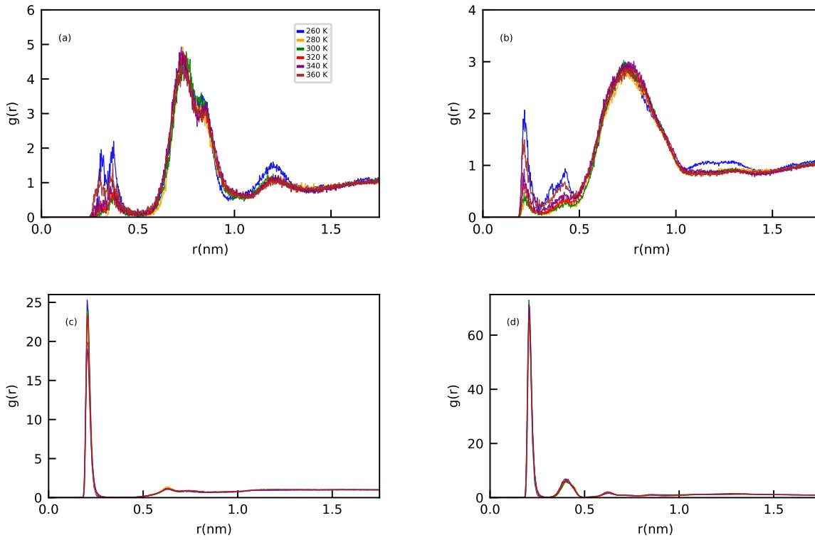
**Figure S11:** Radial distribution functions of (a)  $\text{Li}^+$ -P, (b)  $\text{Li}^+$ -F, (c)  $\text{Li}^+$ -O<sub>EA</sub>, and (d)  $\text{Li}^+$ -O<sub>EMS</sub> as a function of temperature. We present the data for temperatures with a difference of 20 K for better visualization.
