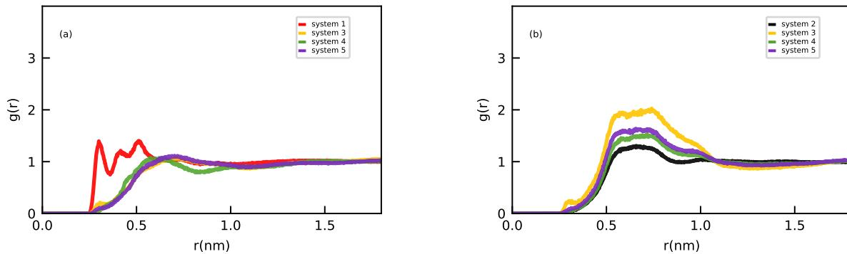
**Figure S3:** Radial distribution functions,  $g(r)$  of (a)  $\text{PF}_6^-$  and oxygen atoms of EA, (b)  $\text{PF}_6^-$  and oxygen atoms of EMS as a function of different molar ratio of EA and EMS.
