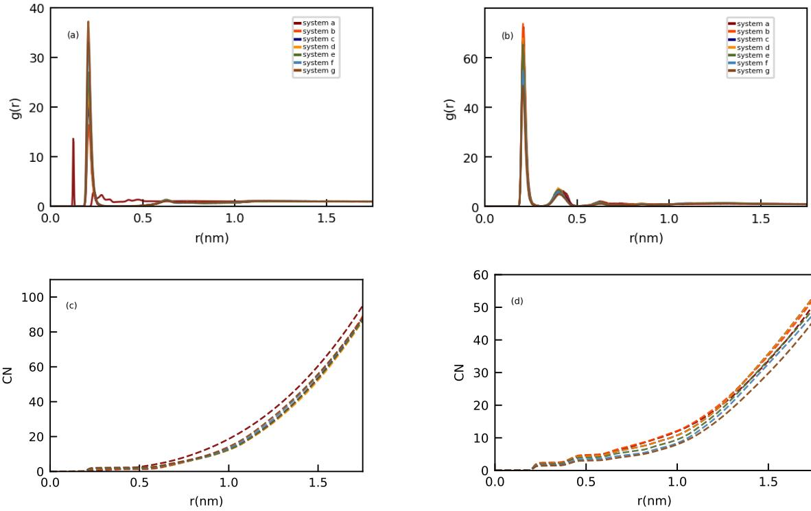
**Figure S8:** Radial distribution functions of  $\text{Li}^+$ -OEA (a) and  $\text{Li}^+$ -OEMS (b) with their integrated profiles, panels (c) and (d), respectively as a function of different salt concentration.
