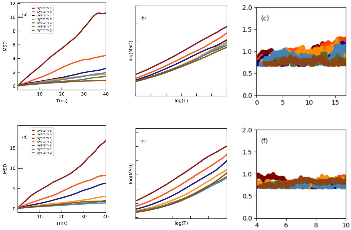
**Figure S10:** Upper panel of figure represents the diffusive motion of cation while the lower panel of figure represents the diffusive motion of anion in systems with different salt concentration. The left panels (a) and (d) represent the mean squared displacement, the middle panels (b) and (e) represent the log MSD versus log T plots and the left panels (c) and (f) show the beta value which corresponds to the diffusive regime.
