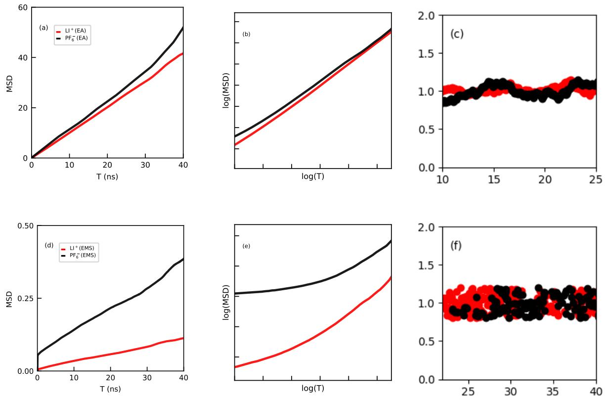
**Figure S4:** The left panels (a) and (d) represent the mean squared displacement, the middle panels (b) and (e) represent the log MSD versus log T plots and the right panels (c) and (f) show the beta value which corresponds to the diffusive regime for the cation and anion in unmixed EA and EMS systems, respectively.
