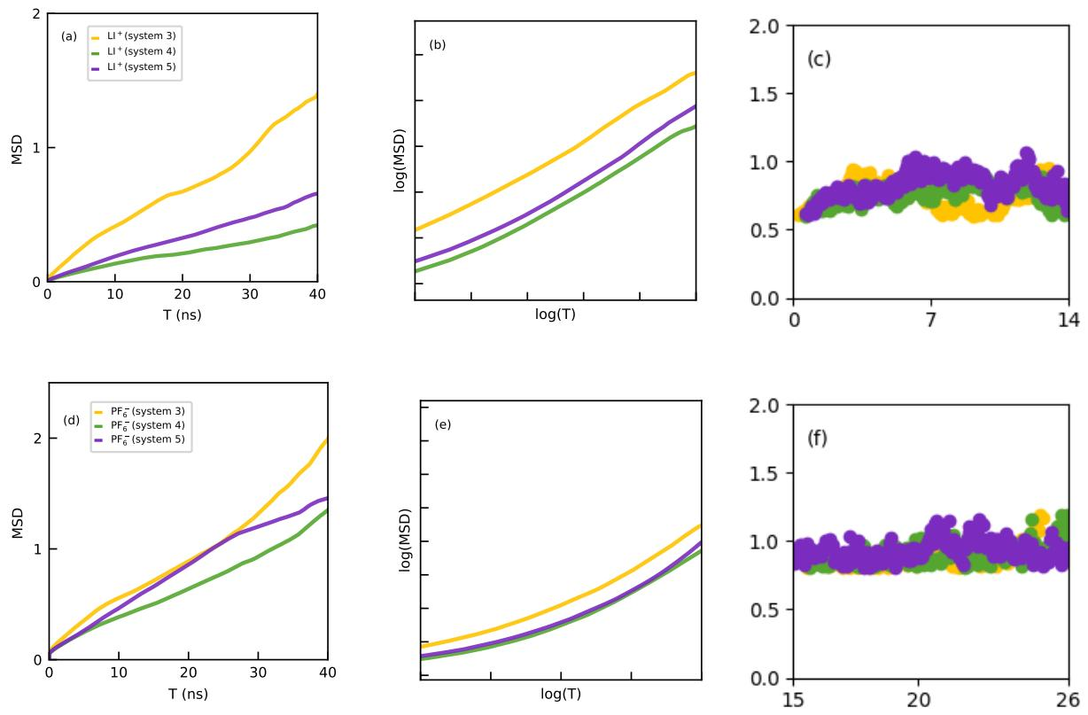
**Figure S5:** Upper panel of figure represents the diffusive motion of cation while the lower panel of figure represents the diffusive motion of anion in different solvent mixtures. (a) and (d) represent the mean square displacement, (b) and (e) represent the log MSD versus log T and (c) and (f) represent the beta value which is shown under diffusive regime.
