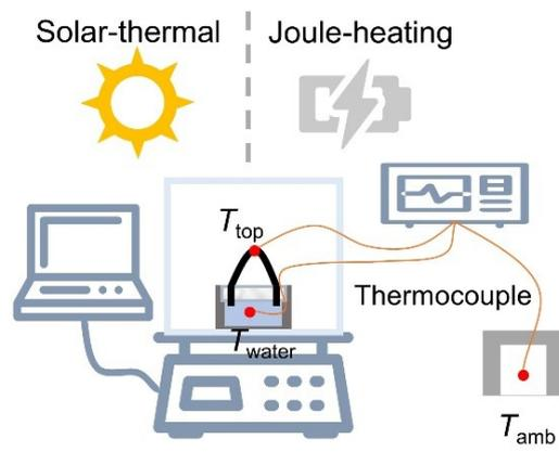
**Fig. S10. Schematic diagram of outdoor experiment setup.**
