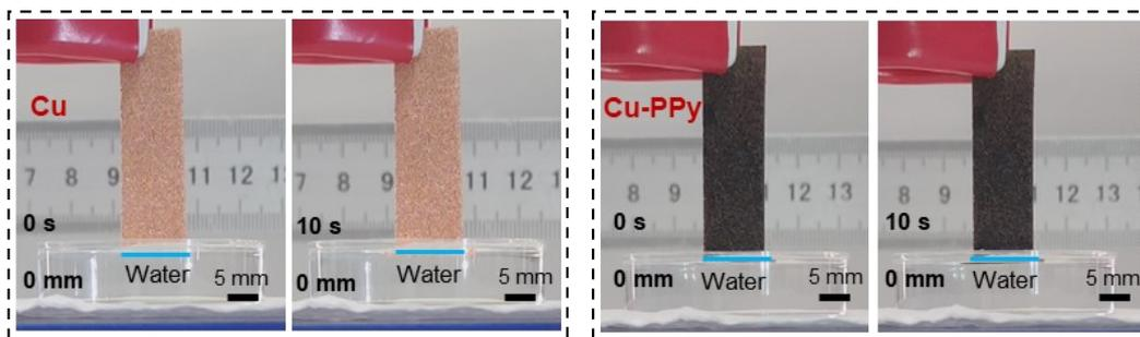
**Fig. S6. Optical picture of Cu and Cu-PPy foam inserted into water reservoir for water supply against gravity.**
