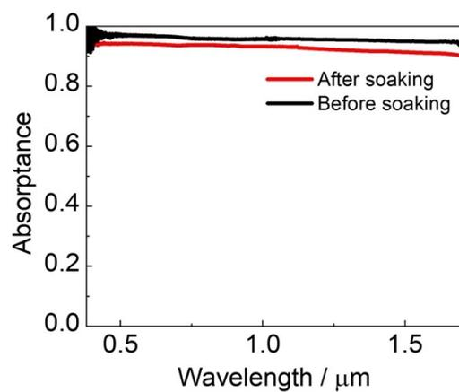
**Fig. S9. Spectral absorbance of Cu/CuO-PPy foam before and after soaking in 10 wt.% brine for 12 h.**
