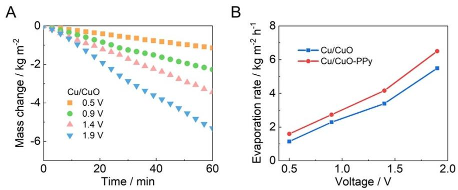
**Fig. S8. Evaporation performance of 3D Cu/CuO evaporators driven by Joule heating at different voltages. (A) Mass changes. (B) Evaporation rates.**
