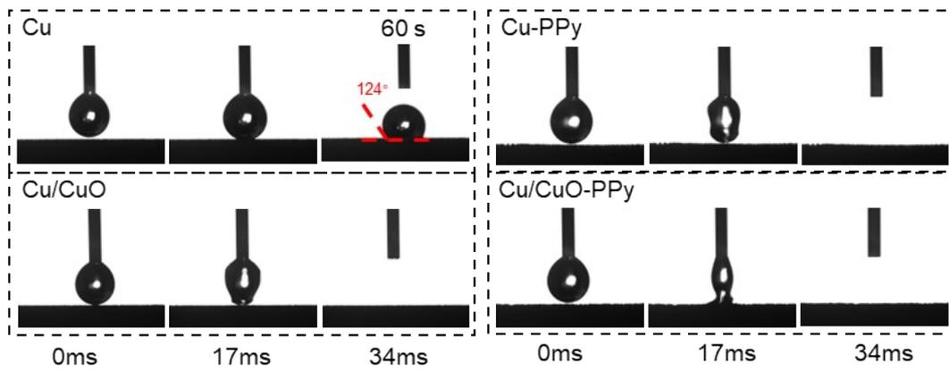
**Fig. S4. Water contact angle variations of different samples.**
