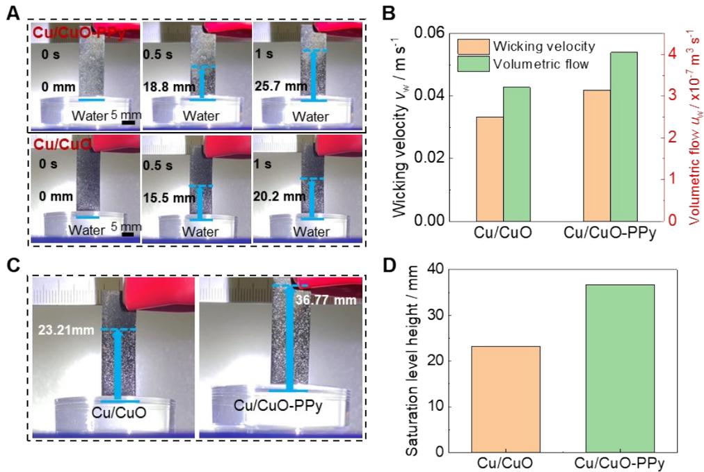
**Fig. S5. Liquid supply (wicking) capability of Cu/CuO foam and Cu/CuO-PPy foam wicking structures.** (A) Snapshots of wicking experiments on Cu/CuO foam, and Cu/CuO-PPy foam. The wicking front is marked by the blue dashed lines; (B) Average wicking velocity  $v_w$  and volumetric flow rate  $u_w$  on the Cu/CuO foam and Cu/CuO-PPy foam; (C) Photos of Cu/CuO foam and Cu/CuO-PPy foam when the water level reaches a stable state; (D) Saturation level height of Cu/CuO foam and Cu/CuO-PPy foam.
