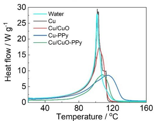
**Fig. S3. Differential scanning calorimetry curves of water in Cu foam, Cu/CuO foam, Cu-PPy foam, Cu/CuO-PPy foam, and pure water.**
