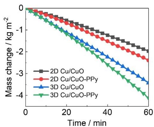
**Fig. S7. Mass change curves of the 2D Cu/CuO foam, 2D Cu/CuO-PPy foam, 3D Cu/CuO foam, and 3D Cu/CuO-PPy foam evaporation systems under 1 sun.**
