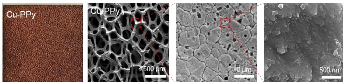
**Fig. S2. Optical picture and SEM images of the Cu-PPy foam.**
