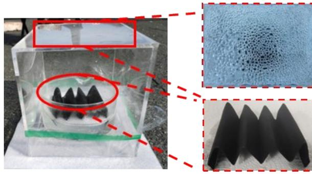
**Fig. S11. Experimental setups for outdoor water yield performance evaluation.**
