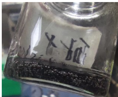
Supplementary Figure 3. Reaction between \text{Li}_{21}\text{Si}_5 and polar solutions.
