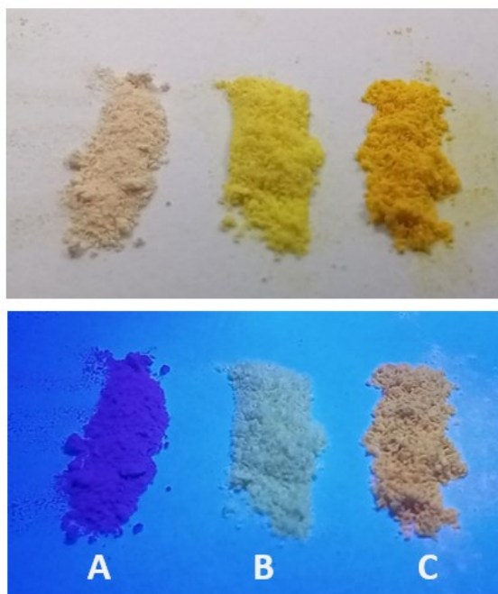
Figure S3 Powder samples of PIM-EA-TB (A), PIM-BTZ-1% (B) and PIM-BTZ-5% (C) without (top) and with (bottom) UV-illumination.
