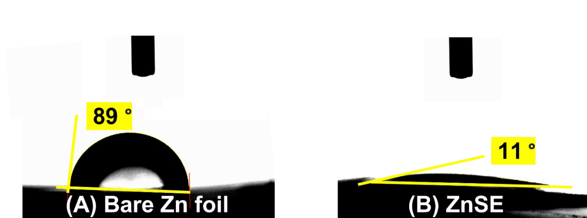
Figure S4. Contact angles of deionized water on the surfaces of the bare Zn foil and ZnSE.
