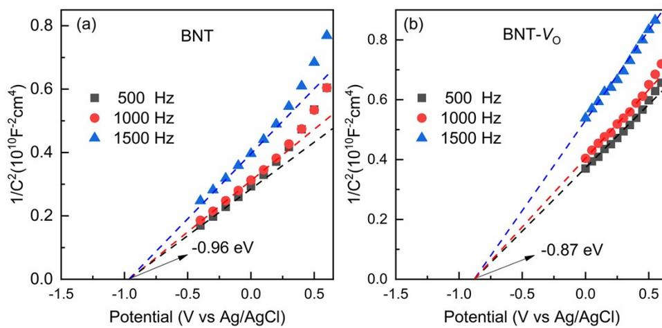
Fig. S6 Mott-Schottky plots of (a) BNT and (b) BNT- $V_O$  at frequencies of 500 Hz, 1000 Hz and 1500 Hz.
