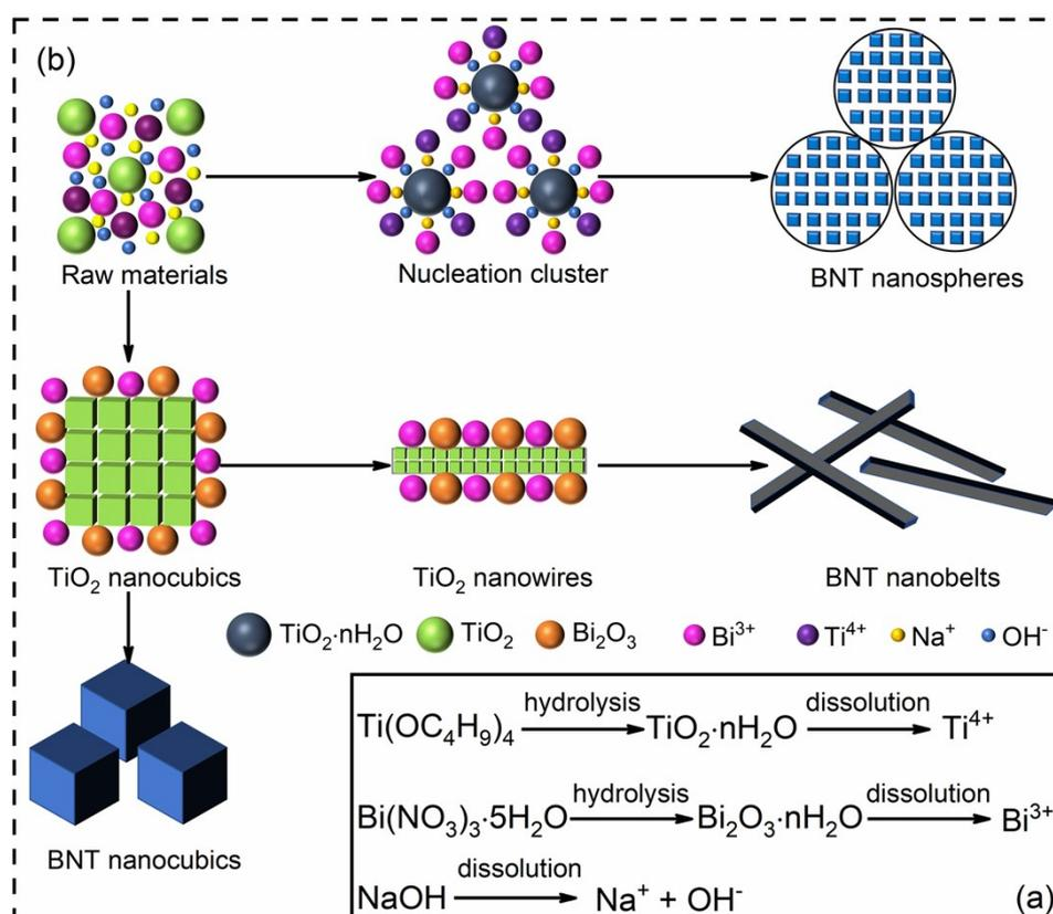
Fig. S4 Schematic of the formation mechanisms for BNT-based nanoparticles and nanobelts.
