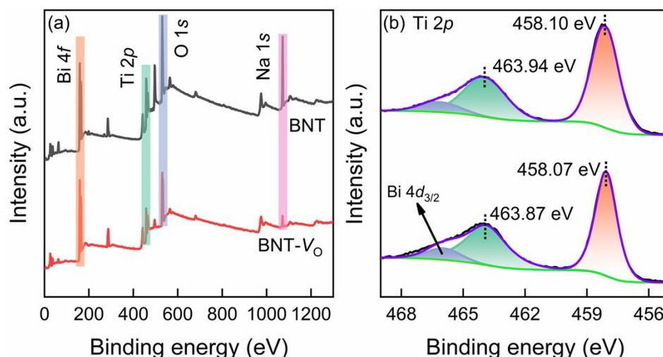
Fig. S1 (a) XPS spectra containing the four constituent elements survey scan. (b) Ti 2p XPS spectra.
