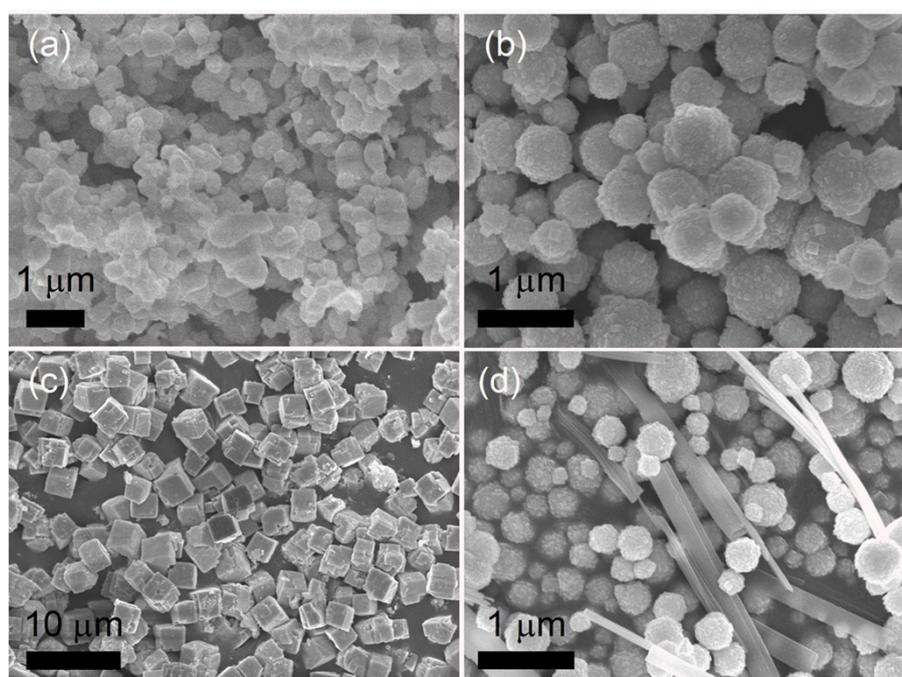
Fig. S3 SEM of different morphologies of BNTs: (a) Bulk, (b) Sphere, (c) Cube and (d) BNT.
