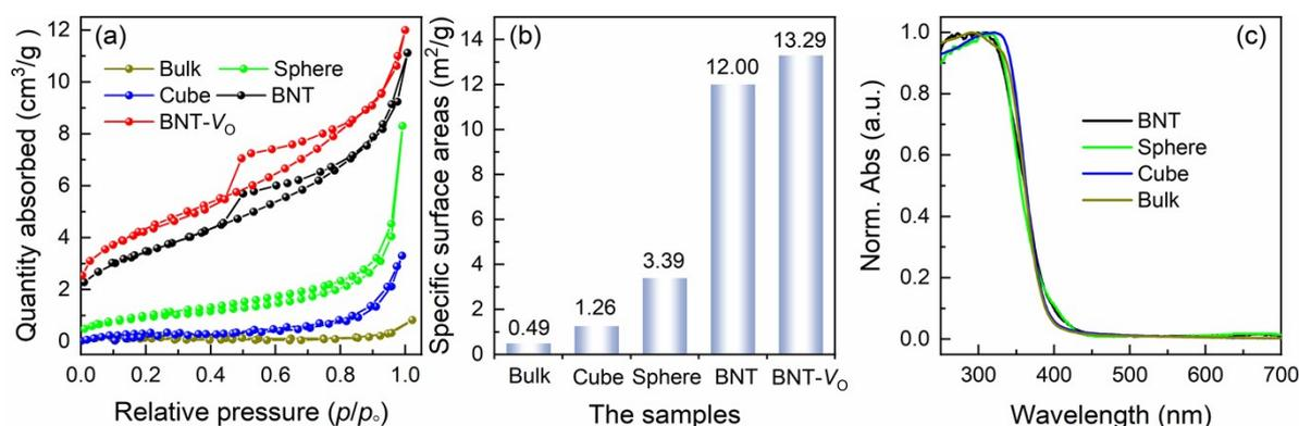
Fig. S5 (a)  $\text{N}_2$  adsorption isotherm and (b) corresponding specific surface area of Bulk, Sphere, Cube, BNT and BNT- $V_0$ . (c) UV-vis spectra of Bulk, Sphere, Cube and BNT.
