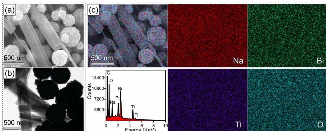
Fig. S2 (a) FE-SEM, (b) TEM and (c) EDS mapping of BNT.
